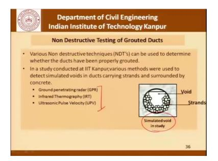
Moving forward the next thing that I wanted to share with you is some tests which are carried out after the grouting operation has been completed, and that work was carried out here at IIT Kanpur and that something which is of interest was, these were the 3 methods which were used to check if a simulated void in the duct could be located After the grouting operation has been completed. The test were ground penetrating radar infrared thermography and ultrasonic pulse velocity.
