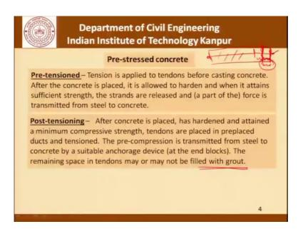
Now, prestressing is done in 2 ways. One is called pre tensioning, where tension is applied to tendons before casting the concrete and after the concrete is placed it is allowed to harden. And when it attains sufficient strength the strands are released and a part of this force is transmitted from steel to concrete. Typically railway sleepers and so
