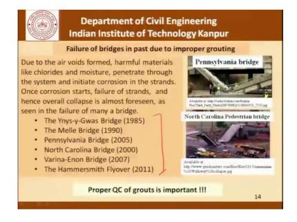
Now There have been reported failures in the past due to improper grouting this is the list of recorded bridges in flyovers which have known to collapse and the collapse is been attributed to corrosion in the strands which has been attributed intern to faulty grouting practices the quality control in the grout and therefore, we must be careful and ensure proper quality control in grouting. I invite you to take a look in the literature and find out more about the failure in these bridges.
