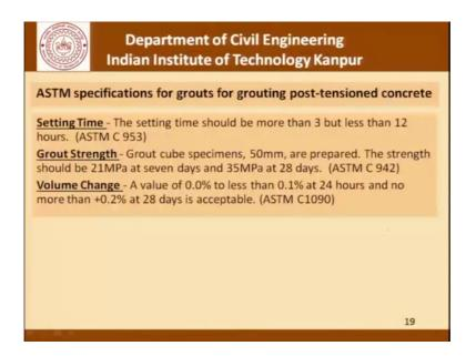
Continuing with the discussion on ASTM specifications for grouts for grouting post tension concrete the setting time should be more than 3 hours, but less than 12 hours the grout strength using 50 mm cubes should be 21 Mpa at 7 days and 35 Mpa at 28 days and volume change is as given here.
