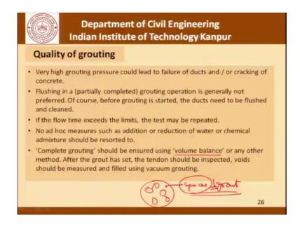
So, as far as the quality of the grouting is concerned we are not talking of the grout we are talking of grouting now a very high grouting pressure could lead to failure of ducts and or cracking of the concrete surrounding it.
