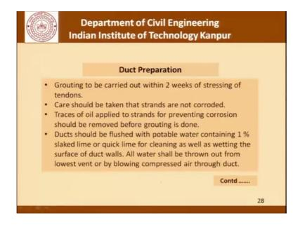
As far as duct preparation is concerned grouting to be carried out within 2 weeks of stressing the tendons we cannot leave the tendons on grouted if that is what is the design for more than 2 weeks care should be taken that strands are not corroded traces of oil applied to strands for preventing corrosion should be removed before the grouting is done.
