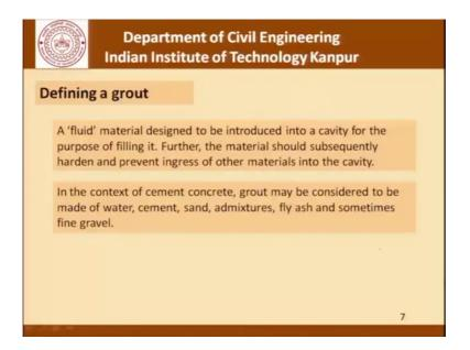
Now, defining a grout a fluid material designed to be introduced into a cavity for the purpose of filling it is; obviously, what is called a grout. Further the material should subsequently harden and prevent ingress of other materials in to the cavity. In the context of cement concrete grout may be considered to be made of water cement sand and admixtures fly ash and sometime very fine gravel.
