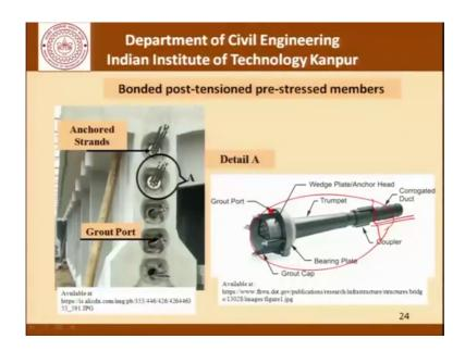
This Picture here shows you a completed I girder where we have anchor strands the grout port and this is the entire assembly which we use before the duct. So, there is the duct
