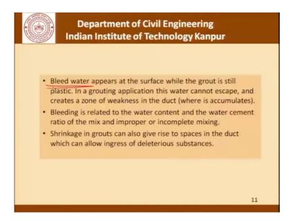
Continuing with our discussion let us try to understand now some of the issues which are involved bleed water appears at the surface while the grout is still plastic. In a grouting application this water cannot escape and creates a zone of weakness in the duct. So, we can imagine that after all there is a certain amount of water that bleeds to the surface of the grout.
