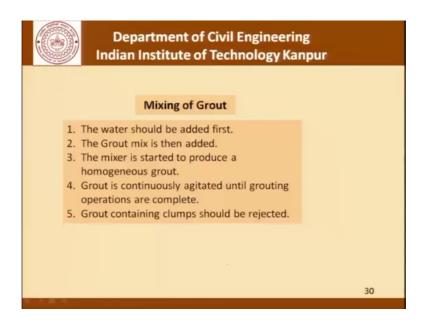
As far as mixing is concerned, the water should be added first the grout mix is then added the mixer is started to produce a homogeneous grout, grout is continuously agitated onto the grouting operations is complete and any grout containing clumps must be rejected.
