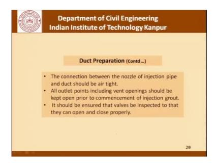
And continuing with the preparation, the connection between the nozzle of the injection pipe and duct should be air tight all outlet points including vent opening should be kept open prior to commencement of the injection of grout. And it should be ensured that valves be inspected So that they can open and close properly.
