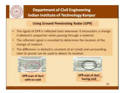
So, these are the Results from the ground penetrating radar system and we find that the GPR scan of the duct having voids is different from that which is seen in the case of ducts which have no voids. Of course, the application and the interpretation of this data requires certain amount of expertise in handling GPR systems.
