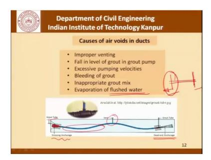
And let us move Forward and try to understand how we get air voids in ducts and avoiding this air voids is the prime concern as far as good quality grouting is concerned.
