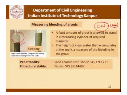
As far as bleeding is concerned is a very simple test of fixed amount of grout is allowed to stand in the measuring cylinder of required diameter. And the height of clear water that accumulates at the top is a measure of the bleeding in the grout the ground is basically a paste it has only cement and water plus of course, maybe some admixtures.
