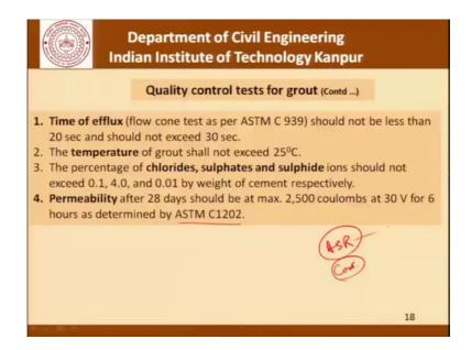
Continue With these qualities there is the time of efflux which could be measured using a flow cone test as per ASTM C 939 and that should not be less than 20 seconds, but should not exceed 30 seconds.
