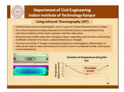
This is the result from the infrared thermography and this is the result from ultrasonic pulse velocity studies.
