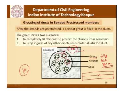
Now, grouting of bonded prestress members after strands are prestressed the cement grout is filled in the ducts this picture at the bottom is a schematic sketch of what I was drawing earlier. So, there is concrete here that is outside the duct, this is the duct casing this strands inside this and the grout which is feeling the remaining space in the duct between the boundary and the strands.
