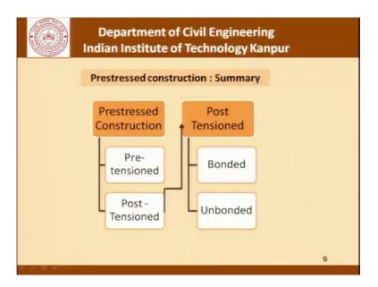
So, to summarise There are 2 types of prestressed concrete construction one is pretensioned and the other is posttensioned and within the posttensioned there is the bonded and unbounded construction. So, once we have this picture in mind we are ready to get started with our discussion on grouting.
