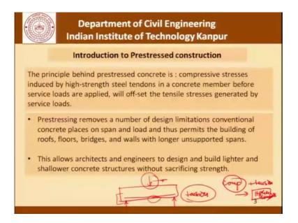
Now, is an introduction to prestressed concrete the principle behind prestressed concrete is compressive stresses induced by high strength steel tendons in a concrete member before service loads are applied will offset the tensile stresses generated by service loads. Basically the principle is very simply understood in the contest of a beam that if you have a beam which is like this let us say it is a reinforced concrete beam which is subject to a load, the part here is subjected to tension.
