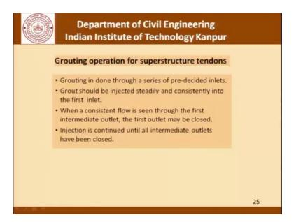
Now, as far as the operation is concerned the grouting is done through a series of predecided inlets. The grout should be injected steadily and consistently into the first inlet and when a constant flow is seen through the first intermediate outlet the first outlet may be closed injection is continued until all intermediate outlets have been closed.
