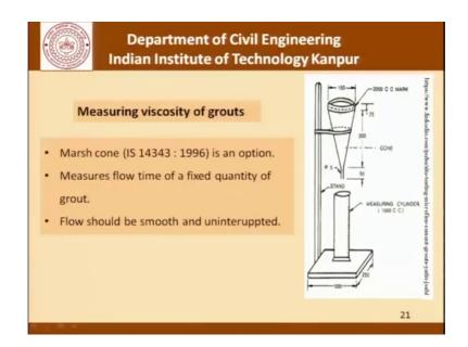
Now, this is a schematic representation of measuring viscosity of grouts using let say the marsh cone you must ensure that the flow smooth and uninterrupted.
