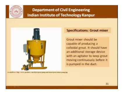
These are the specifications for the mixer and these are the Specifications for the grout pump.
