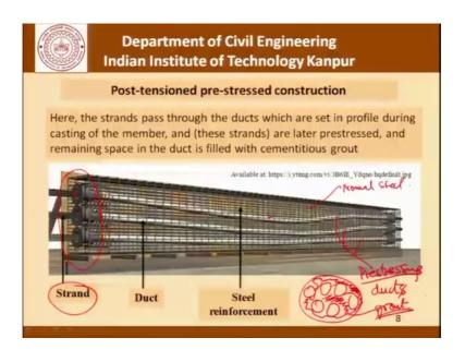
Now, this picture I think would make the whole process very clear. This shows how posttension prestress construction is done. The strands pass through the ducts which are
