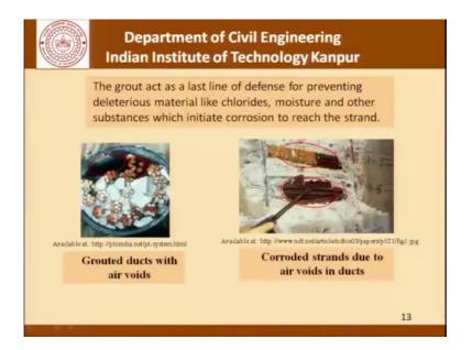
Now, the Grout act as the last line of defence for preventing deleterious materials like chlorides moisture and other substances which initiate corrosion to reach the strand. And here are pictures of what could go wrong we can see in the picture on the left hand side that there are places where the void has not reached. And if this happens of course, we will have corrosion in the ducts. And that is something which we want to definitely avoid.
