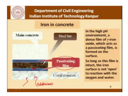
And the reason for that is that there is this passivating film that forms on the reinforcing bar. And this acts as a barrier for any kind of deleterious material that may enter from the outside in reaching this surface.
