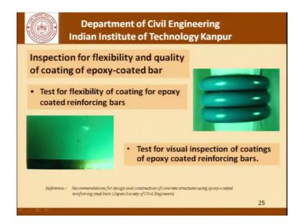
As far as flexibility and quality control of the coated bar is concerned that has also to be a flexibility test of the coating for the coated bars. And visual inspection for the coatings of epoxy coated reinforcing bars. So, these extra deposits of epoxy should also be avoided to the extent possible. And depending on the severity or the frequency of occurrence of these defects the bars may be accepted or not accepted for a particular application.
