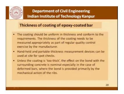
Moving forward we must know the thickness of coating of the epoxy coated bar, they should be a bend test which needs to be carried out because reinforcing bars are often required to be bent in their applications in beams columns and so on.
