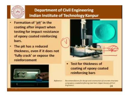
So, this is that kind of cup that forms and what we are interested to know is if this deformation or the damage is such that if we use this kind of a device, which is similar to that which is used for detection of pin holes will that device cause or detect a contact. So, of course, the voltage that we are using need not be exactly the same as we use for the case of pin hole detection.
