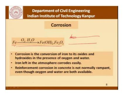
A work about corrosion basically iron going to oxides and hydroxides in the presence of oxygen and water is what corrosion is, and this process has to happen on the surface of the steel. So, if we have a steel bar in order that this bar corrode at the surface somehow this process of iron going to it is oxides and hydroxides should happen. Having said that we must note that reinforcement corrosion in concrete is not normally rampant even though oxygen and water are both available.
