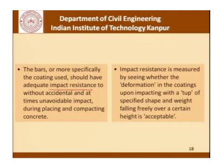
Moving forward as far as impact resistance is concerned the bars are indeed exposed to impact resistance it could be during the handling or it could be even during placement of concrete when we are using vibrators which will; obviously, hit sometimes the reinforcing bars inside. And the impact resistance is measured by seeing whether the deformation in the coatings upon impacting with a tup of a specified shape and weight falling freely over a certain height is acceptable.
