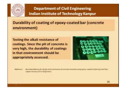
So, this here is a view of the epoxy coated bars being tested in actual concrete they are embedded cured and tested as far as their durability and their suitability for a particular concrete environment is concerned.
