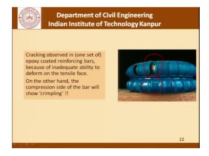
So, this is the kind of breaking or cracking in the coating that is going to be formed whereas, in a good bar that will not happen. So now, this testing; obviously, has it is own set of parameters including the diameter of this ruler about which the bend is to be made.
