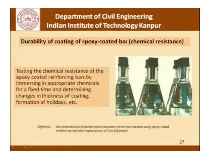
The chemical resistance is to be tested by using high pH and possibly solutions having some amount of chloride to ensure that the epoxy coated bars are such that they can withstand the kind of chemical environment that they are likely to encounter once they are inside concrete.
