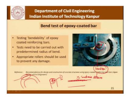
And this bendability of bars is an important test because once we bend these bars the outer surface here is subjected to tension. And if the coating which is there on the bar is not able to sustain the tension or the tensile strains, what we will have is what is shown here.
