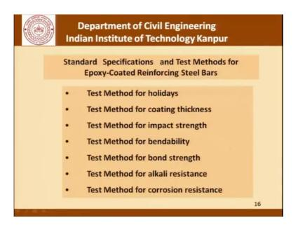
So, moving forward as far as testing is concerned for quality these are some of the methods or some of the tests that are required. Testing for holidays, coating thickness, impact resistance, bendability, bond strength, alkali resistance and corrosion resistance. Now obviously, for each of these tests or each of these properties we need to have a specific test methods.
