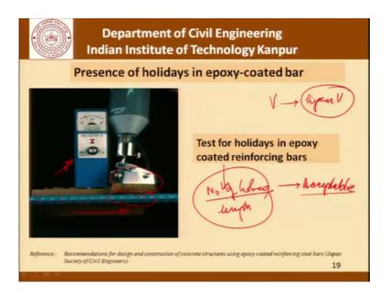
This here is a picture showing the testing for holidays and this is the device this is our meter that we talked about and we are trying to determine if there are pin holes or holidays in this region. It is obviously, to detect the holes at different locations. So, this hand held device is moved along the length of the bar and we try to find out if there are any holes anywhere.
