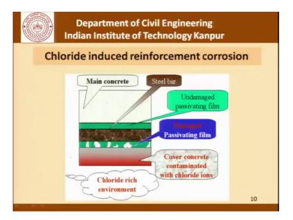
So now, this passivating film can be damaged; however, if what is getting into the concrete is something like chlorides. Now these chlorides have the property of attacking this passivating film kind of eating it away making this part let us say here or this part somewhere here vulnerable to corrosion and that is where corrosion gets initiated.
