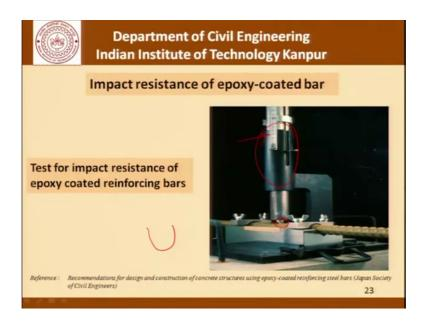
Now, as far as impact resistance is concerned we have discussed it before. This is the semispherical tup and it is mounted on this vertical support with a graduated scale and as it falls on the reinforcing bar what we get is a situation like this where the coating has been damaged.
