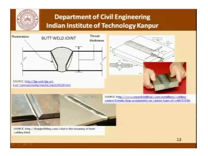
Similarly, there are issues related to the butt welding and this picture here shows a butt welded joint. Similar pictures of butt welded joints are given here.
