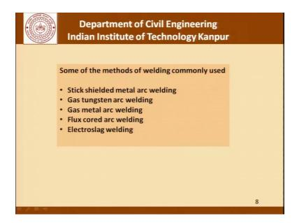
Some of the methods of welding which are commonly used are: stick shielded metal arc welding, gas tungsten arc welding, gas metal arc welding, flux cored arc welding, and electro slag welding.
