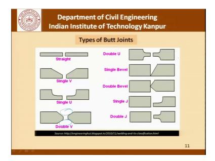
So, moving forwards this picture here gives you the different types of butt joints: single V, single U, double V. So, you can see that we are trying to divide these types of joints depending on how much and where is the material being deposited, and also what kind of edge preparation we do as far as getting the joint ready is concerned.
