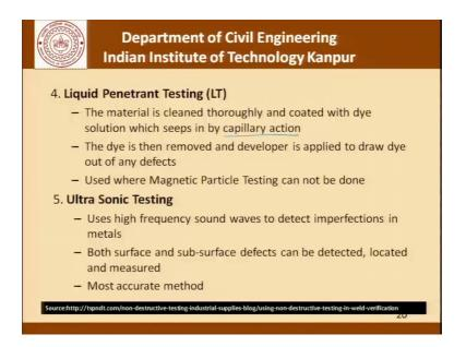
Next in the line of testing of welds is liquid penetrate testing which is called LT. The material is cleaned thoroughly and coated with dye solution which seeps in by capillary action. Here again we are trying to understand if here is any capillary action as a result of pores or defects in the weld. The dye is then removed and a developer is applied to draw the dye out of any defects and used where magnetic particle testing cannot be done.
