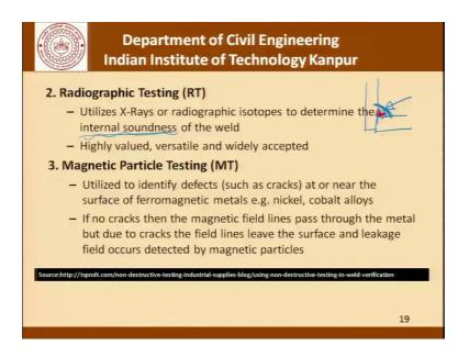
Coming to the radiographic testing which is the next step utilizes X-Rays and radiographic isotopes to determine the internal soundness of the weld. Now here we are talking about internal soundness which is simply not possible to inspect through a visual inspection. If we recall the picture of a fillet weld for example or it could be any other
