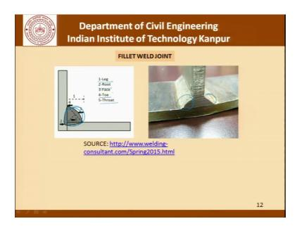
So, this here shows a picture of a fillet weld and we see that this is the material which is been deposited: and in welding terminology we call a leg, root, face, toe, and throat. So, as far as the stress transfer is concerned the structural engineers know as to what kind of stresses act when it comes to a welded area here which will be subjected to shear stresses, and how they are computed, what is the shear strength of the weld, and so on.
