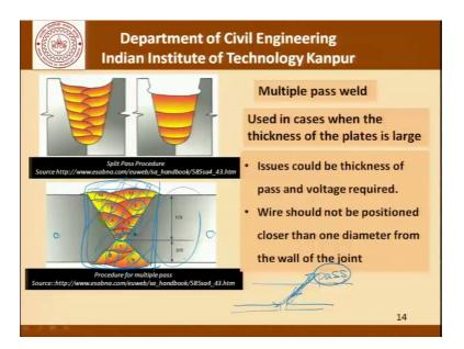
And then I must introduce to you the concept of a multiple pass weld. What this multiple pass weld is it is used in cases when the thickness of the plates is very large and we cannot deposit the material in a single pass.
