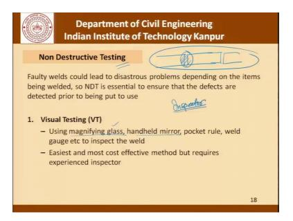
So, even though that is not our subject primarily, but it is interesting and it is important for us to know some of the tests which are commonly used for non-destructive testing of welds. Faulty welds could lead to disastrous problems depending on the items being welded, so non-destructive testing is essential to ensure that the defects are detected prior to the system being putting used.
