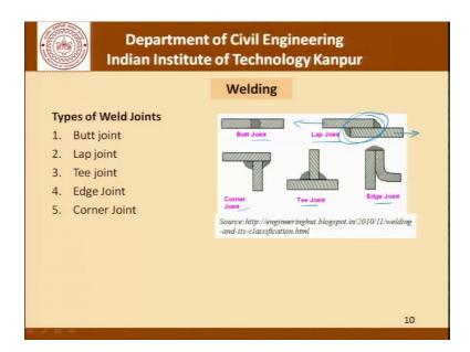
These are some of the common welding types that we use in structure engineering, in civil engineering, butt joints, lap joints, tee joints, edge joints, and corner joints, and you can see how they look like. The butt joint here, it is a lap joint, a tee joint, edge joint, and a corner joint. Of course, as structural engineers we know that if we do joints like this it introduces certain eccentricity as far as a transfer a force is concerned.
