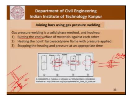
Now, what this method does is not use traditional welding. In traditional welding there is a material here, and there is a material here we do some kind of edge preparation here. We have an electrode that deposits additional material and we get a weld. As far as gas pressure welding is concerned it does not involve deposition of additional material. What it does is that the 2 ends of the bars are butted against each other, we make sure that the
