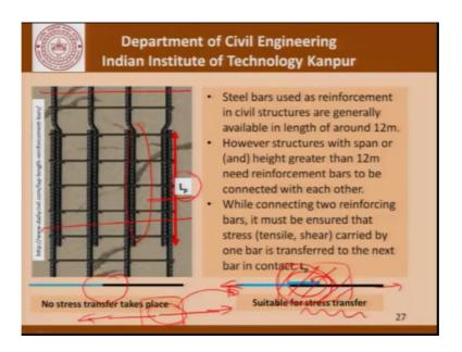
We will continue our discussion today and look at another very simple issue when it comes to concrete construction. That is lapping or splicing of reinforced concrete bars when it comes to RC construction. So, a steel bars used in reinforcement in civil structures are generally available in lengths about 12 meters.
