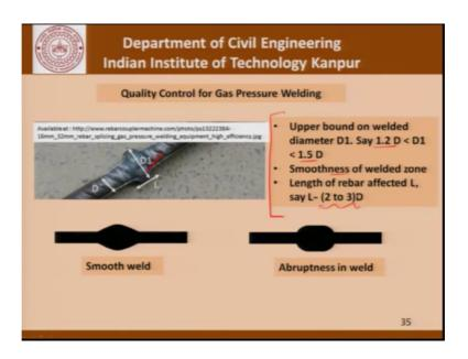
This picture here shows how the gas pressure welding is carried out. You can see this wise here which is there to hold the bar together one end of the bar and the other end of the bar is here. And this is specially designed flame burner which is heating the joint across for a certain length. And finally, what we get is a gas pressure welded joint which would
