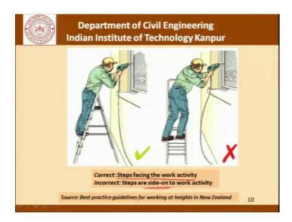
Similarly if we see this slide, here also is an example of the right way of working with ladders and the wrong way of working with ladder. Facing directly towards the steps, facing the work activity and steps being side on as far as the work activity plane is concerned makes a lot of difference when it comes to safe working with ladders.
