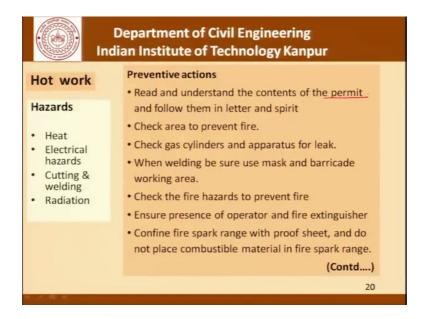
Moving forward let us talk about what is called hot work in the construction industry and hazards in this area would be heat, electrical hazards, cutting and welding and radiation. A kind of preventive action that we talk about in these conditions would include read and understand the contents of the permit and follow them in letter and spirit. I would like to
