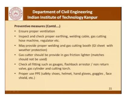
We must ensure proper ventilation inspect and check proper earthing, welding cables, gas cutting, hose machine, regulator and so on, may provide proper welding and gas cutting booth which could be made with a GI sheet with weather protection. That basically says that in the site, we isolate an area provide a lot of the right infrastructure in that area, but
