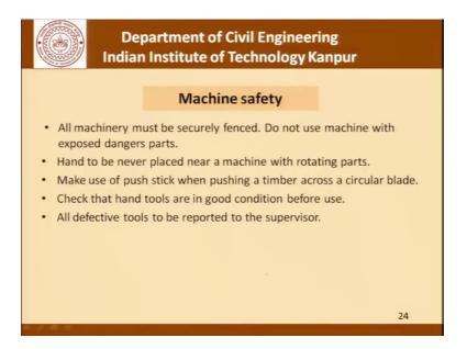
Another special condition as far as construction sites is concerned is the use of machines. We cannot live without using machines at a construction site and we have to observe certain precautions. All machinery must be securely fenced. So, that they do not fall do not used machines with an exposed dangerous parts. Hands should never be placed near a machine with rotating parts whether it is a peddles to fan or any such machine.
