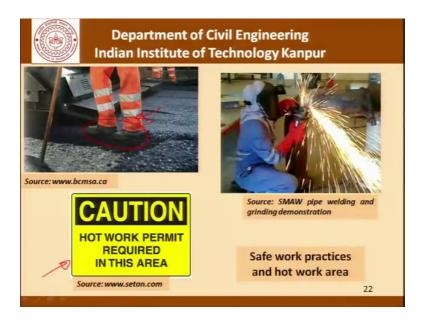
And these pictures here show you two examples of hot work; in one case you are talking of bituminous construction and another case we are talking of pipe welding and grinding and we can see a lot of sparks flying around. So, you can imagine that these sparks pose a major hazard as far as fire is concerned and effort needs to be made to confine these sparks to a local area.
