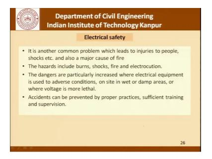
It is another common problem which leads to injuries to people, shocks and it also a cause for fire, the hazard includes burns, shocks, fire and electrocution, the dangers are particularly increased where electrical equipment is used in adverse conditions. For example, if the site is wet or in damp areas where the voltage requirement is lethal, Accidents can be prevented by proper practices, sufficient training and supervision.
