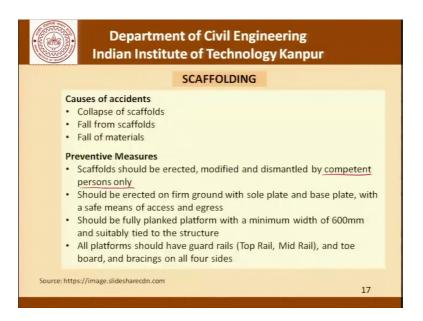
So, moving forward let us talk of Scaffoldings the Causes for accidents is for as scaffolding is concerned could be the Collapse of scaffolds, Falls from scaffolds, and Fall of materials of the scaffold. And some of the Preventive Measures would be there should
