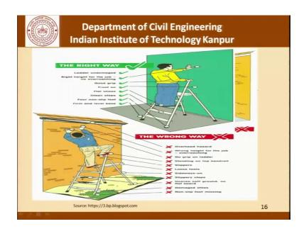
This picture here is of course, a Cartoonists way of looking at the right way of using the ladder and the wrong way of using the ladder. We can see that this person here is trying to work on a wall not facing the wall which leads to a very avoidable unnatural position for doing the work and is a safety hazard as for as the ladder is concerned.
