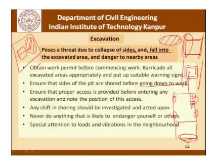
Excavation poses a threat to the collapse of sides, and fall into the excavated area, and danger to nearby areas. As for as the collapse of sides is concerned the explanation is simple that if we excavate this area, whether this sides should be vertical, or they should have a certain slope, depends on the type of soil, depends on the depth of excavation, whether the soil is wet or dry the groundwater table and so on.
