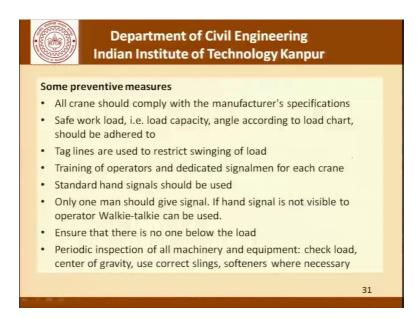
As far as some preventive measures as far as crane failure is concerned; all cranes should comply with the manufacturers, safe work load capacity angle according to the load chart should be adhered to.
