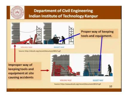
These are examples of Proper and Improper ways of keeping tools and equipments at construction sites. We see here that the site is, so much more clean and this place is a cluttered site; a cluttered site is a very very difficult site to navigate and is the cause for accidents.
