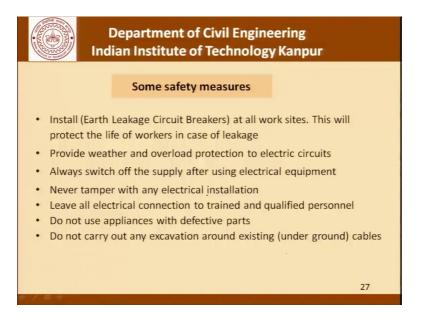
So, some of the safety measures that we can take is installation of earth leakage circuit breakers at all work sites and this will protect the workers in the event of a leakage. Provide weather and overload protection to electric circuits, always switch off the supply after using electrical equipment, never tamper with any electrical installation, leave all electrical connection to trained and qualified personnel.
