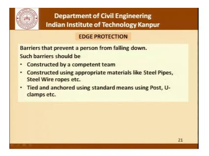
So, moving forward let us talk a little bit about edge protection Barriers that prevent a person from falling down is what edge protection is and these barriers should be Constructed by a competent team, and Constructed using appropriate materials like steel pipes, steel wire ropes and so on. And Tied and anchored using standard means such as posts, U-clamps etcetera.
