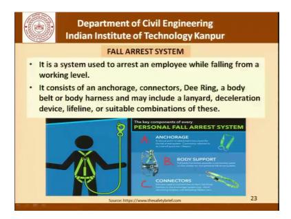
So, moving forward this is one of the examples of the fall arrest system, which is used to arrest in employee while falling from a working level it consists of an anchorage, connectors, Dee ring, a body belt or body harness, and may include a lanyard, deceleration device, lifeline, or a suitable combination of these.
