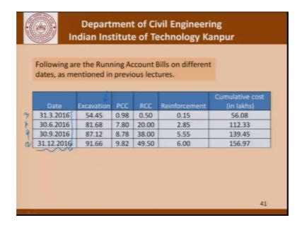
Now, in addition to this total cost we also had information about the work that had been completed at the end of 3 months, 6 months, 9 months and 12 months and this was indeed the completion of this project and the value of the excavation, PCC, RCC and the reinforcement work which had been arrived from the quantities of the work done at the different points and time. So, now, this was the cumulative cost of billing or the cumulative value of the work at different points in time.
