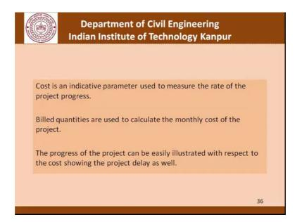
So, value of work done is an indicative parameter used to measure the rate of the project progress billed quantities that is the work completed used to calculate the value of the work done on a monthly or a cumulative manner and the progress of the project can easily be illustrated with respect to the cost or the value of work done showing and it also shows the delay if it is occurring in that project.
