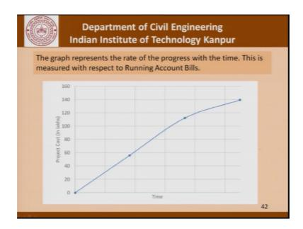
So, if this now was to be plotted on a graph we will get a curve something like this which is precisely the S-curve that is precisely the plot of the project which shows how the total value of work done has changed with time. This picture of course, does not really show the characteristics of the S-curve except towards the end and in the initial part we find that the value of the work done is much higher.
