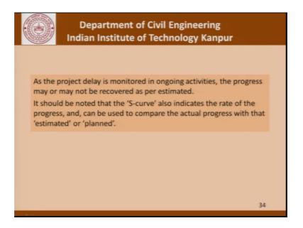
As the project delays monitored in ongoing activities the progress may or may not be recovered as planned. So, it should be noted that the S-curve also indicates the rate of the progress and can be used to compare the actual progress with that estimated or planned.
