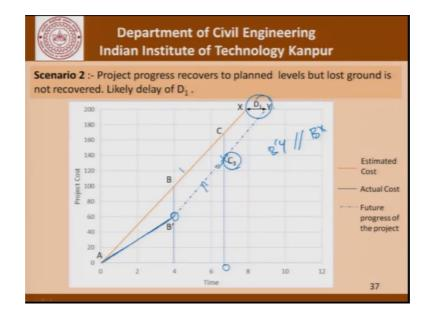
Instead of that if you are working in a manner that well the progress at the initial parts was lower than what was planned, but from this point onwards we will come back to a slope which is the same as this in another words B dash Y is parallel to B X then what we are looking at is a delay of D 1 and in that case at the same point of monitoring we are working against a value of C 3.
