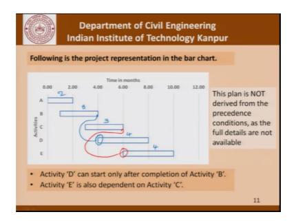
So, this is the bar chart representation of the 5 activities - A starts at 0 goes for to two which is 2 months, B starts at 1 and goes on till 4 which is 4 months and C is also 3 months D and E are 4 months each. So, what we are showing here is that this project completion is in 10 months.
