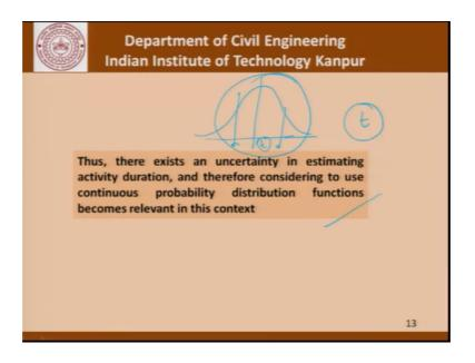
This underlines the need to understand that there exists an uncertainty in estimating activity duration and therefore, considering to use continuous probability distribution functions becomes relevant in this case. So, what we are saying in this sentence is instead of assigning a particular time t for any activity can we now talk in terms of a probability distribution, that is yes this activity will take some time, but that time could be may be
