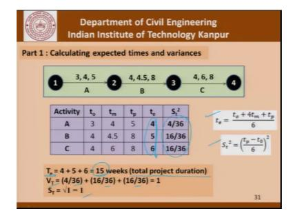
So, moving forward we first calculate the t es and the S t squares using this formulae and we found out the capital T which is the total project duration by summing up these three small t es and we find 15.
