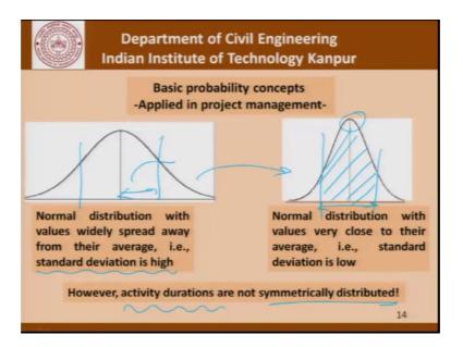
The normal distribution with values widely spread away from the average is the situation where their standard deviation is high. Compared to this picture this picture here is a situation where the peak is sharper which means that the area in this part is closer to the mean, if you want to go to the same area here we will go more standard deviations away from the mean; however, in both cases the normal distribution is symmetric.
