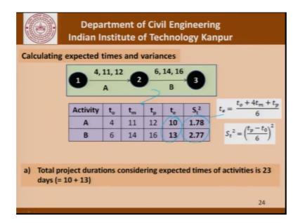
So, working out the t e and the standard deviations we find that for activities A and B we convert this information to this table here the using these formulae we calculate the expected times of completion of the activities and the variances. So, the total project duration considering the expected time of the activities is 23 that is 10 and 13.
