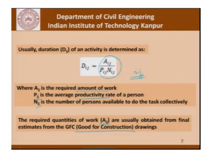
Going back to the basics usually the duration D ij of an activity is determined using this formula which is A ij upon P ij multiplied by N ij, where ij is the activity that we are talking about. A ij is the required amount of work, P ij is the productivity of the person which could possibly take care of the learning curve and so on, and N ij is the number of persons working on that job independently and together.
