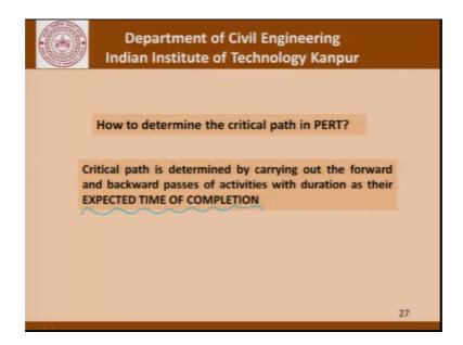
So, continuing our discussion further how do we determine the critical path in this method? The critical path is determined by carrying out the forward and backward passes of activities with durations being taken as the expected time of completion. So, of course, we take the expected time of completion and then we use probability concepts too find out what are the probability of completing the project in that time and so on.
