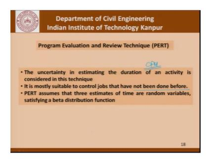
Pert is the program evaluation and review technique and the uncertainty in estimating the duration of an activity is considered in this technique as against the critical path method that we saw in the last class where the activities had a firm time of completion. It is more suitable to control jobs that have not been done before and there is more uncertainty in the activities.
