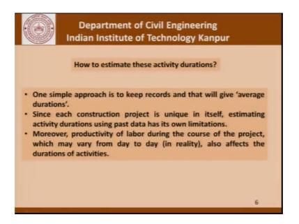
One simple approach is to keep records that will give us the average durations. So, a construction company keeps a record for erection of process and so on and finds out that in different projects what is the kind of time that it takes and from there we try to find out the productivities and then try to map that into a new project and try to estimate the time involved for that project.
