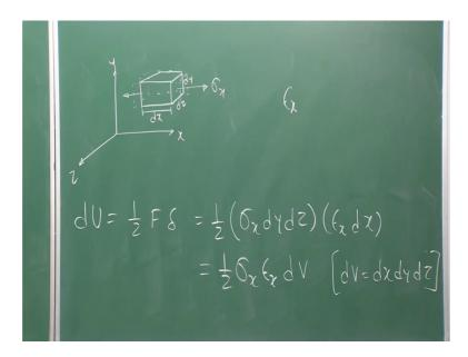
Now, we are considering one infinite similarly small element within a linear elastic body in the previously we have considered that we know in when we are talking about the stress distribution of stress and all. So, we are considering what infinite similarly small element inside a inside an elastic body. And that is nothing but like this.
