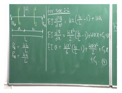
For section 2 2, E I d 2 v d x 2 is equal to bending moment, that is M b for section 2 2, please try to remember. So, that already we have calculated W x B by L minus 1 plus W a.
