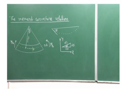
The moment curvature relation. So now, as you recall so, this is so, this was your neutral axis. So, this is the beam after bending. And see this angle which is made at the centre say phi. And the radius of the curvature say rho. And this is under pure bending situation will be already we have seen that thing earlier pure bending situation say.
