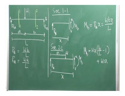
The problem is like this very simple problem we are taking to understand this thing in a bitter way. You have a simply supported beam reaction R A and R B. So, this is point A point B you have one concentrated force W here, which is acting at a distance away from a and this is B the total length of the beam is say L and fine.
