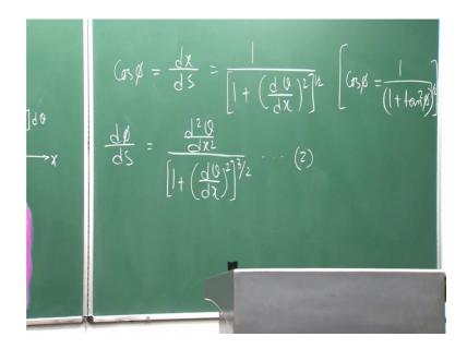
Which can be written as 1 by 1 plus d v d x whole square to the power half. So, where from where this is this relation is coming this is simple geometrical relation, because as you know cos phi from your trigonometry 1 by 1 plus tan square phi to the power half. That you know right. From trigonometry relation this thing is known to me ok.
