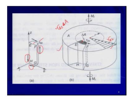
So, what is your equilibrium requirements because you are applying the twisting moment and that twisting moment is causing the development of this shear stress right.
