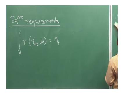
So, this shear stress is nothing, but the internal say adjustment this internal force shear force which is developed at each cross section that will try to balance the externally applied twisting moment M t right. So, that we are getting from this figure. So, here actually what you are getting you are getting tau theta z acting on the plain. So, this is one this the say cross sectional plain. So, therefore, to balance as you know. So, cross
