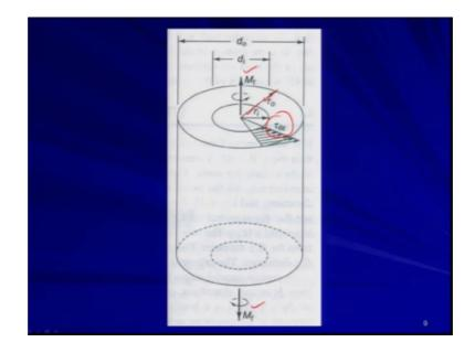
Now, for this hollow circular shaft your I z is simply equal to as we have calculated 2 minus pi r i to the power 4 2 right that gives me 1 minus r i to the power 4 r o to the power 4. Now what you are getting from this actually, your polar moment of inertia for a hollow circular shaft is given by this expression fine.
