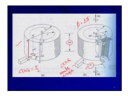
So, now if we look at this shear and if we try to analyse the prior diagram, if you look at this figure this figure the bottom section actually this is one segment we are taking one segment from the circular shaft and this is the say depth of the segment delta z fine. Now what I am saying the rotation of after due to the application of the twisting moment the oration of the bottom section is say phi which is the say initially it was here and after that it is going here right.
