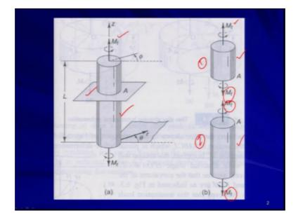
Now, if you consider this kind of say circular shaft, so for the time being, we are considering the solid shaft. And this shaft is basically under the action of the torsional moment M t, the circular shaft loaded only by twisting moment M t at its ends at both ends you are having M t that means, you are having a circular shaft you are giving the
