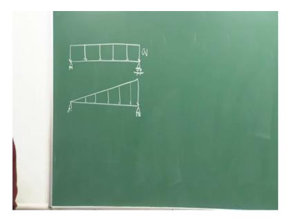
Then how it varies, it either it varies constantly either the distributed load say this is the beam either you have this kind of distributed load constant distributed load with constant load intensity q per unit length or you may have this kind of loading linearly varying loading. So, generally most of the times will be using or will be dealing with this kind of distributed load now if you have this kind of distributed load how you will analyze the
