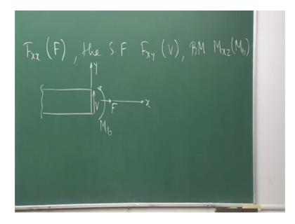
So, in the z direction; that means, normal to the beam is very unuseful. So, in that situation you have only three components left out to define the nature of slender member. What are those? Fx x that is nothing, but the axial force, the shear force F x y that will be defined as v and bending moment that is M x z and that will be called as Mb. So, if I considered this is my slender member, this is my say x direction and this is y.
