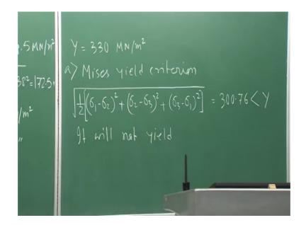
So, the in the problem it is said that y value is equal to, that y is equal to 330 sorry 330 mega newton per meter square. Now, as per misses yield criterion half sigma 1 minus sigma 2 whole square plus sigma 2 minus sigma 3 whole square plus sigma 3 minus sigma 1 whole square right. So, that is coming as 300.76 which is less than y.
