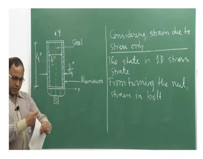
So, total depth of the arrangement is 4 inch. So, this is your aluminum sleeve all round aluminum sleeve something like your cylinder, inside that you have the steel nut and this is the bolt sorry steel bolt and this is the nut and this total outer dimension is 3 fourth inch and the inner dimension is 1 half inch. So, we are we are solving this thing this problem in aps unit whenever less that is not a problem well.
