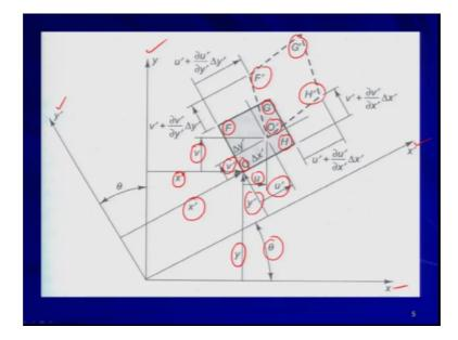
So, now if you look at this figure the basically this is your x y coordinate system. Now, we are going to define the state of strain in x prime y prime coordinate system which is oriented with respect to the angle theta and that means, the angle between the x prime
