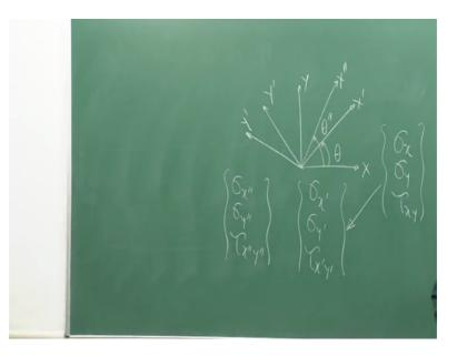
So, what did I mean? Suppose this is your x y coordinate system this is your x y coordinate system. Now, another coordinate system you are considering say x prime y prime which is making this is known to me which is making an angle say theta with respect to x axis now I know the state of stress in x y coordinate system; that means, I know sigma x sigma y and tau xy.
