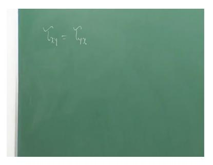
So, if you get the cross shear which are equal then basically the 9 components will come down to 6 components basically right. So, you need 9 stress components to define the state of stress at a point already we have seen in the last lecture.
