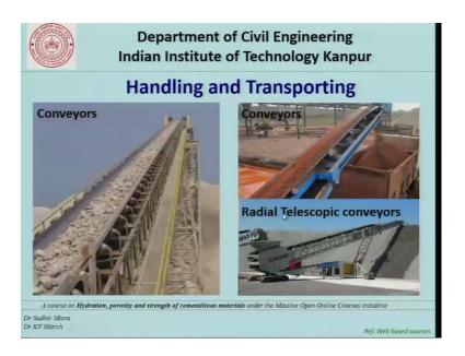
In addition to these you also have handling and transporting equipments like conveyors bills conveyors. So, here you can see that the material or feed from one location in the plant to another location in the other case one location to dram truck and like vice you also have telescopic conveyors which can actually increasing in length if the distance to convey the material is more.
