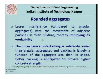
In addition rounded aggregates have lesser interference compare to angular aggregates with the movement of adjacent particles in fresh mixture thereby improving its workability. So, from workability stand point rounded aggregates or largely preferred their mechanical interlocking is relatively lower than angular aggregates and packing is largely a function of the aggregates size than its shape better packing is anticipated to provide higher concrete strength.
