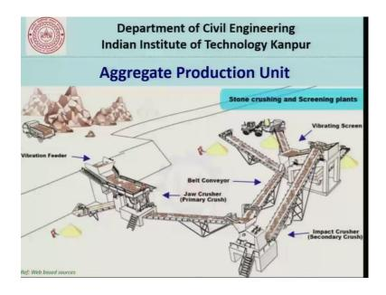
So, in the figure what you see is a aggregate production unit in one side, you have the natural resources available in the form of rocks and in the other side you have the aggregate production unit which is usually install very close to the aggregate source. So, the aggregate production unit consist of vibration feeder primary crusher secondary crusher some belt conveyors vibrating screens and also you have some stock files and we will see each one of them in detail.
