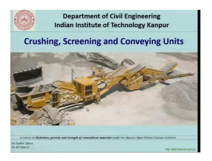
So, in this figure, what we see is a crushing screening and conveying unit all club together. So, all that you can see is that bigger rocks or feed here and they are basically broken down in a primary crusher unit and it is taken over by some conveyer bills and some screen are available to divided into a specified particles size and finally, you see that they are stored in stockpiles.
