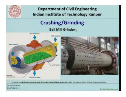
In addition to the primary and secondary crushing sometimes ball mill grinders are also used, but remember that ball mill grinders are primarily used to make the particle size to
