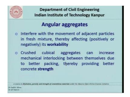
In addition angular aggregates interfere with the movement of adjacent particles in fresh mixture thereby affecting its workability remember workability can be positively affected or negatively affected and that again depends on several other factors crushed cubical aggregates can increase mechanical interlocking between themselves due to better packing thereby providing better concrete strength.
