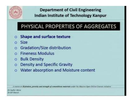
So, the physical properties of aggregates plays a very important role now the different physical properties of aggregates include shape and surface texture size gradation or size distribution fineness modulus bulk density, density and specific gravity water absorption and moisture content in this lecture we will see only about shape and surface texture in other lectures we will see the remaining part.
