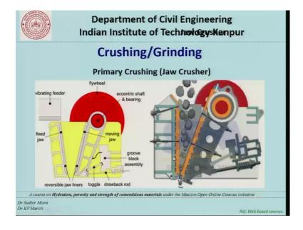
Now, the second one is crushing or grinding and in that what we see is that we have something called as primary crusher and the jaw crusher or very often use for primary crushing and here you have two figures to the left you have the figure without aggregate feeder it. So, the primary crush essentially consists of a fixed jaw more or less vertical and you also have a moving jaw which is inclined some angle. So, that the spacing at the bottom is lower compare to the spacing at the top.
