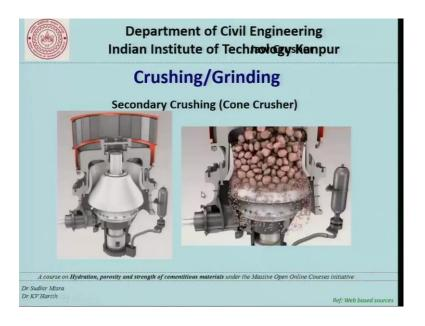
In the second case, we have secondary crusher one example of secondary crusher is cone crusher where you have a cone that is rotating at some angle this part receives the aggregate and the rotation of the cone basically crushes the aggregated into finer parts. So, in this figure what you see is the coarse aggregate that are feed from the top and because of the revolution of the cone.
