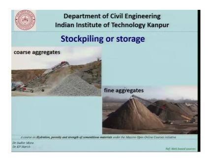
So, once you get the aggregates of different sizes they are actually kept in stockpiles and later on dram trucks come to the aggregate production plant and take it to the site where the construction is performed. So, in this figure you see the coarse aggregate piles and in the other figure you see the fine aggregate piles.
