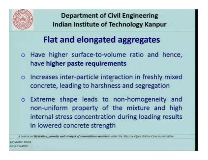
So, from the stand point of packing and from the stand point of strength angular aggregates or generally preferred compare to other aggregates now flat and elongated
