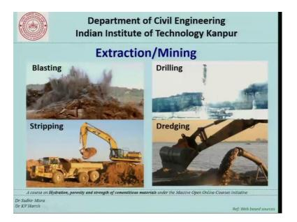
Now, the figure here shows the blasting operations drilling operation stripping operations and dredging operation as you can see that depending upon the hardness of rocks each of these operations or carried out if the rocks are hard a nature then blasting and drilling operation may be require if the source of rocks or softer in that case here you have soft material stripping is used if the aggregate sources or delay water bodies in that case the process of dredging is used.
