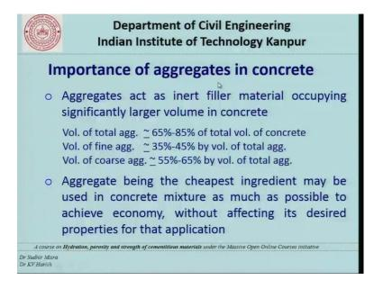
Now, what is the important of aggregates in concrete aggregate act as inert filler material occupying significantly larger volume in concrete volume of total aggregate is approximately 65 to 85 percentage of the total volume of concrete volume of fine
