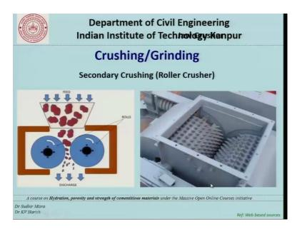
You also have another type of secondary crushing unit called as roller crusher in which two rollers or fixed at some distance and the aggregate or feed from the top; obviously, the spacing this much higher at the top and because of the roller the aggregate materials or broken down into finer particles this is the typical figure of a roller crusher.
