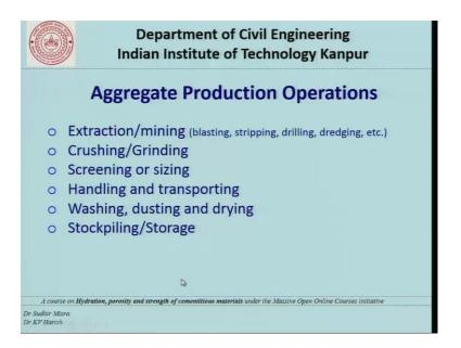
So, aggregate production operations include the following extraction or mining crushing or grinding screening or sizing handling and transporting washing dusting and drying stockpiling or storage in extraction or mining usually blasting stripping drilling or dredging operations or perform.
