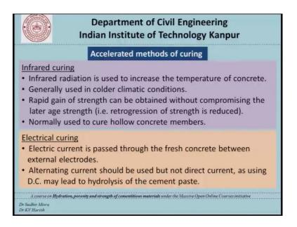
Continuing with methods for accelerated curing there is infrared curing which means infrared radiation is used to increase the temperature of concrete generally used in colder climate conditions, rapid gain of strength can be obtained without compromising the lead age strength and normally used to cure hollow concrete members.
