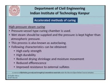
In this case there is a pressure vessel type curing chamber and we use wet steam and pressure is kept higher than atmospheric and this process is also known as autoclaving. The following characteristics can be obtained if we use this autoclaving curing process high early strength, high durability, reduced shrinkage and moisture movement, reduce the efflorescence improved resistance to external sulfates and so on.
