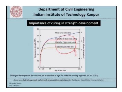
This picture again is also something which we had seen last time and we can clearly see that depending on the conditions that the concrete has after the initial period the strength could be very different.
