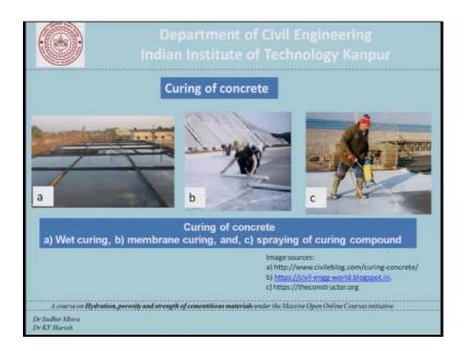
These pictures here show wet curing membrane curing in the spraying of curing compounds. So, we can see that in the situation like this we have the luxury of being able to pond simply pond the surface of a slab and indeed of course, this water evaporates into the atmosphere and is lost. So, from the water conservation point of view indeed this is not a very effective method of curing even though from a concrete standpoint this perhaps the best that we can do when trying to cure a slab.
