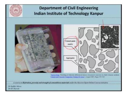
The concrete consisting of aggregate phase and the cement paste matrix and through thus curing process we are essentially trying to ensure that the cement paste matrix indeed develops into a very dense structure where as much as possible of the calcium silicate hydrates are formed and we have as lower porosity as we possibly can get.
