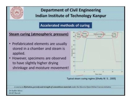
Discussing this whole idea of steam curing a little bit this picture here shows the cycle that is followed there is a delay period, a heating period, a maximum temperature period and then a cooling period. So, all these times have to be carefully decided depending on the type of cement and the type of product, the type of strength that we want and so on.
