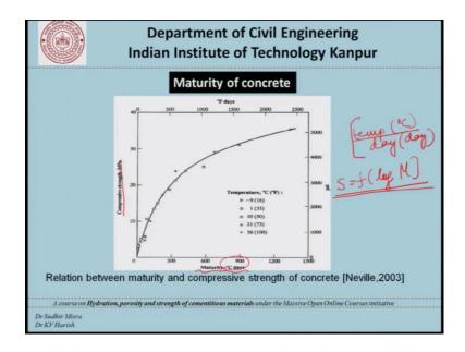
This picture here shows some of the experimental data which is for maturity in degrees centigrade days; so obviously, the unit of maturity will be something like degree centigrade days because we are talking about the product of temperature which is being measured in degree centigrade and the days of curing which will be in terms of days. And this product is maturity related to the compressive strength and we can find that there is a fairly good fit in this relationship.
