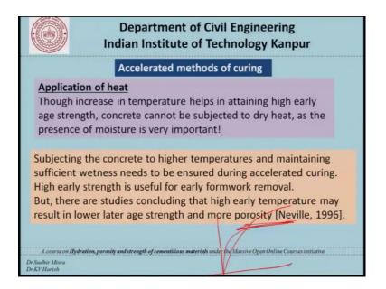
Moving further there are other methods such as application of heat. We must remember that though increase in temperature helps in attaining high early strength concrete cannot be subjected to dry heat as the presence of moisture is very important to ensure the right kind of hydration and strength development. Subjecting the concrete to higher temperatures and maintaining sufficient wetness needs to be ensured during any accelerated curing.
