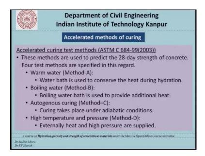
Accelerated curing methods as prescribed in the ASTM 684-99 these methods are used to predict the twenty eight day strength of concrete. Now this is a slightly different viewpoint on accelerated curing. Here the idea is that we want to accelerate the curing with the intent to get an early assessment of the strength that we would get with 28 day cubes or cylinders.
