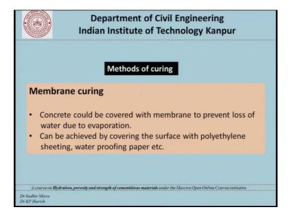
Then there are other methods such as membrane curing. Now what happens in this case is concrete could be covered with a membrane to prevent loss of water due to evaporation this can be achieved by covering the surface with a polyethylene sheet or waterproofing paper and so on.
