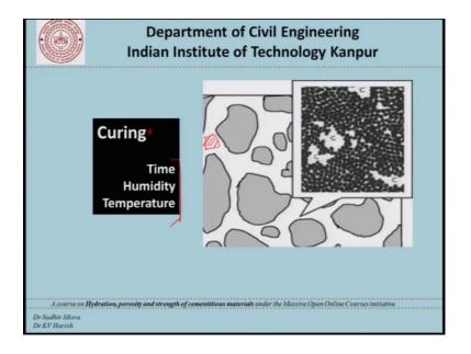
So, when we are talking about curing there is the time of curing, there is the humidity or the conditions that have to be maintained around the concrete and it is the temperature at which the concrete has been cured. These are the kind of things that come to mind. Basically we have to study how these three things or how the curing process affects the hydration or continued hydration that is taking place in this part of our concrete.
