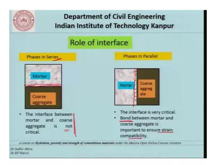
Now, let us talk about the interface, at the end of it the mortar and the coarse aggregate are not necessarily monolithic. The coarse aggregate particles are only suspended in mortar and if we look at the role of this interface, when the phases are in series if we say that well there is an interface in between what is the importance of that interface.
