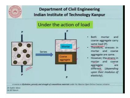
Now, if you look at the action of this concrete which is the real concrete, under the action of load when the phases are in series what we will have is a system like this. Now basic physics tells us that in this case both the mortar and the coarse aggregate will carry the same note, having said that the stresses in the mortar and the coarse aggregate will be the same.
