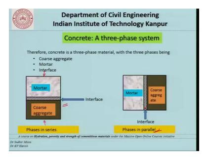
We can therefore, more or less come to a conclusion, that concrete is a three phase material with three phases being coarse aggregate mortar and the interface itself.
