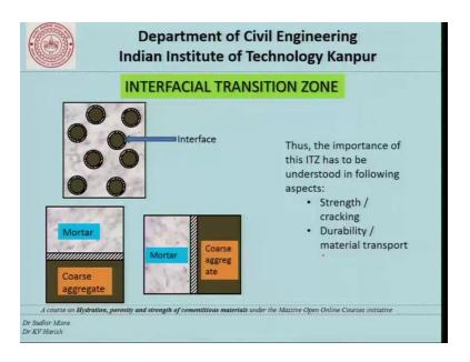
To summarize: the importance of this ITZ can be understood in the following aspects. One is strength and cracking and the second is from the point of view of durability and material transport.
