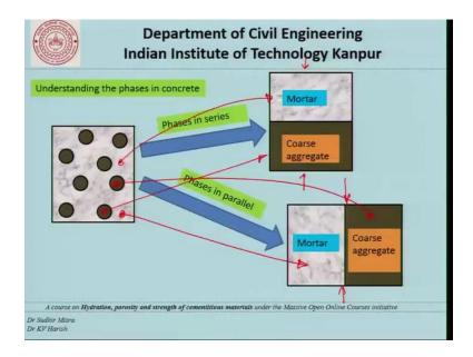
Now, if we what to look at this modeled more closely, we can model at as series representation where we will say that from a load application point of you if the load is being applied like this. All this mortar here is lumped at one place shown here and all this coarse aggregate here is lumped at one place that is shown here. And these 2 phases are a series as for as the load application is concerned. Another representation could be when the phases are in parallel.
