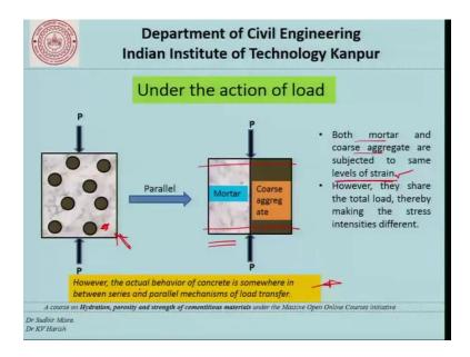
If we take the situation now when the 2 phases are in parallel, then the load carrying mechanism suggests that both the mortar and the coarse aggregate will be subjected to the same level of strain. That is, they have to deform to the same level. And now if the level of deformation which is the strain is the same then the load that they carry which is related to the stress will be different.
