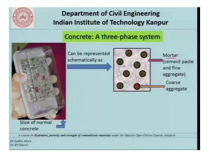
So, let us take a look at this picture which we solve the first lecture, as well which is basically a photograph of what concrete looks like on the inside. We can schematically represent this as coarse aggregates and mortar in a manner that the coarse aggregates here, which is this coarse aggregate particle or suspended in mortar or cement paste and fine aggregate.
