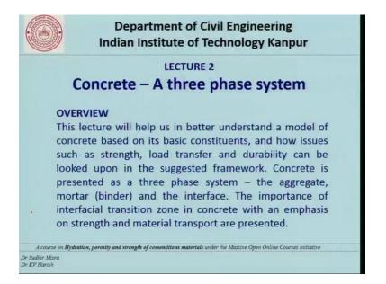
This lecture we will help us in better understand a model of concrete based on it is basic constituents and how issues such as strength load transfer and durability can be looked upon in the suggested framework.
