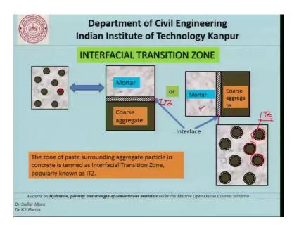
Now, let us look at the interfacial transition zone once again. This is the word model concrete where coarse aggregate particles are suspended in mortar we have this IPZ, which is small zone between the mortar phase and the coarse aggregate phase. In other words, what we have said is that the zone of paste surrounding the aggregate particle in concrete is termed as the interfacial transition zone and is popularly known as the ITZ.
