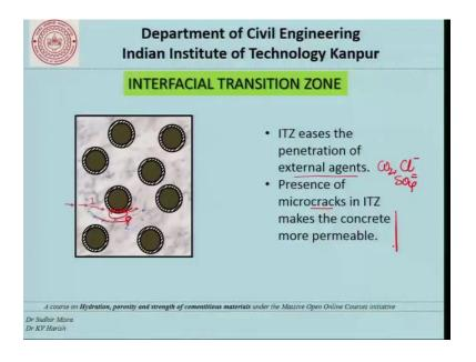
As far as the durability issues are concerned, ITZ eases the penetration of external agents. Basically if the is strength of the ITZ is lower, it is also an indication of the fact that the porosity in the ITZ is higher.
