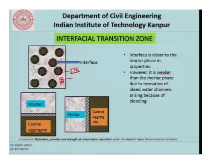
The water cement ratio in the ITZ is slightly higher than that of the main body of the mortar effectively once again the interface is closer to the mortar phase in properties see thus no way that we can argue that this interface between the aggregate particles and the mortar is close to the aggregate, because the aggregate has a very well defined geometry, whereas the mortar is feeling this phase.
