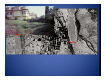
Again without having understanding this structure was been created or built on exactly on the fault, we can see the slide warping here and this is what is the fault scarp, this structure is sitting right on the fault scarp. So next event this structure will definitely go off ok.
