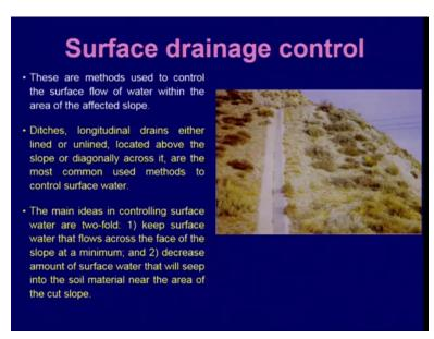
Now surface drainage you can try to construct the drainage on the surface and try to remove or the water as fast as possible because you are not allowing the water to percolate down into the ground okay or on on the slope okay. And that will reduce the the area from having chances of landslides okay. (Refer Slide Time: 20:03)
