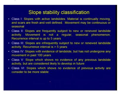
Slope stability if you take, class 1, this may vary from place to place again but in general you can say that slopes with active landslides okay. This is class one where material is continuously
