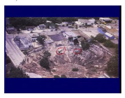
This one is the huge one and you can make out the size of this pothole. This is from US based on the size of this truck here okay, a car here so huge pothole which came up okay because of the subsurface solution activity.
