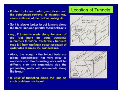
Now location of tunnels if you look at very quickly so we are having a folded structure so the sketch shows your anticline and syncline here okay and then there are two tunnels which are been given here like tunnel A and tunnel B. Now tunnel A is been taken up across the core or it is traveling along the core of the the anticline and here also the B is along core of the anticline and the sands, the rocks which we are having like shale or grate or we say conglomerate okay.
