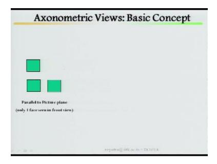
Axonometric views basic concept, look at this parallel to picture plane, what do you mean by parallel to picture plane? A picture plane is there, object is there, it is parallel to picture plane that means only that side, one face you can see, only one face you can see that is your front view.
