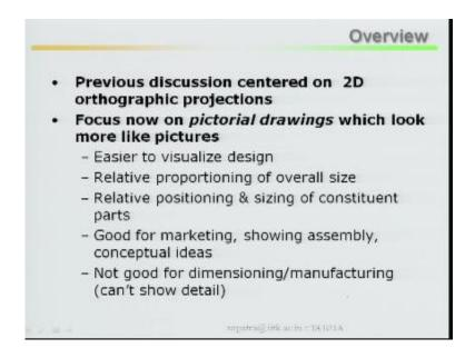
Good for marketing, showing assembly and basically conceptual ideas will be cleared, basic concept will be cleared in this view, not good for dimensioning or manufacturing, not good for dimensioning or manufacturing cannot show the details, cannot show the detail unless if you are not seeing front and top as well as back view you cannot show the details so not good for dimensioning, this is your overview of isometric projections and isometric views.
