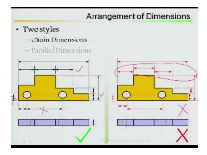
Two styles first one we are talking about chain dimensions, arrangement of dimensions, this is same view same view I am putting it here, look at here left hand side and right hand side. Once you start with the chain dimensioning that means if it starts here it will continue in the same line, if you look at here I am putting it here at the top for this dimensioning, putting at the bottom, here top, bottom, bottom, top, there is no alignment, no alignment.
