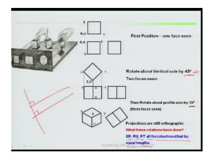
They are, here they are perpendicular with respect to this plane these projection lines are perpendicular, orthogonal with to this, that means still this three views are orthographic, what this rotation have done? If you looked at here rotation have done SR, RU, RT. SR, RU, RT this is your SR, RU with respect to vertical, then RT with respect to profile. All what additional you get it?
