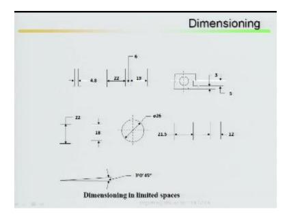
Dimensioning once there is no space is not available you can do this way smaller spacing's, here it is a dimensioning if a 3 degree, zero minute, 45 second, here it is very difficult to do dimensioning inside, here you can make it two arrows then from this arrow you mark it, here you write it three degree, zero minute, and 45 second that means dimensioning in limited space.
