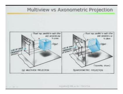
Multi view versus axonometric projections, if you look at here this is your multi view projections hence use line of sight here from infinity that means multiple means you are looking at here, then you are looking at here, then you are looking at here, that means front top as well as side but here you rotate it, you rotate it you are looking at here that means with a single rotations slightly rotating you can visualize three faces.
