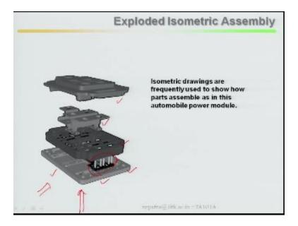
Isometric assembly, as I said simple example, there is a machine assembly, this is your part 1, this is your part2, this is your part3, part 4, part 5. I rotate it in such a way that my viewing direction is in this direction or maybe in this direction it does not matter, rotate it in such a way that standing it here or standing it here I can visualize this side, this side, how the assembly, this part what is its size, is there any hole, is there any notch?
