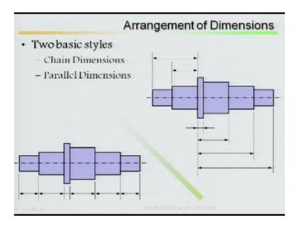
Two basic styles, chain dimensions and parallel dimensions, you can do in a chain dimensioning you can do in parallel.
