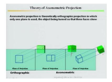
Theory of axonometric projection, what is axonometric projection? Looked at here very carefully, now this is a plane of projection, see there are two views one is this view front view is there in the front view, rear view is there, then there is, here there is a side view is there, this is a plane of projections I am seeing this projection on this plane, come to this, this object has been slightly rotated.
