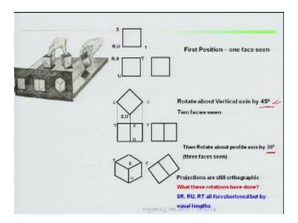
Just see it first position one face in first position one face in, rotate it about vertical axis by 45 degree, this is the standardization, I said you can rotate it at any angle, you can rotate it at any angle depending upon your angle this views will be different views will come. So rotate it about vertical axis by 45 degree. Now this is by 45 degree Q is there, rotate it about vertical axis because this vertical axis here it is rotated about your vertical axis 45 degree.
