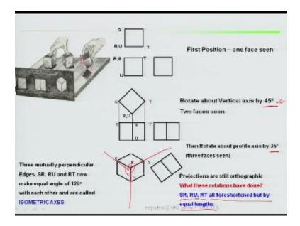
Isometric what are the isometric axes? SR, RU, RT this is your three isometric axes with respect to isometric axes it will be equally foreshortened, that means length, width, and depth that extends it will be equally foreshortened.
