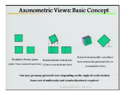
Rotate it about vertical axis as I explained before two slide, two slides before rotate it about vertical axis with respect to vertical axis it has been rotated. I can see two faces in the front view, parallel to picture plane only one face I can see in front view, rotate it about vertical axis I can see two faces in front view. Rotate it about profile axis as I said I can see three faces in pictorial view.
