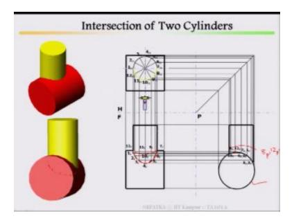
Next example is your intersection of two cylinders. Look at here there is one cylinder, then another cylinder is going inside. I rotate it, rotate it, then how it looks, then take it, finish it top view, this is your top view, this is your front view, this your side view, front view I have not drawn so what happened in the top view? Once you finish the top view outer cylinder mark, inner cylinder how it intersect you mark it.
