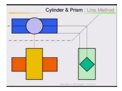
Now let us start with example cylinder and prism by means of lines method. Cylinder and prism, there is a cylinder, intersection between cylinder and prism.
