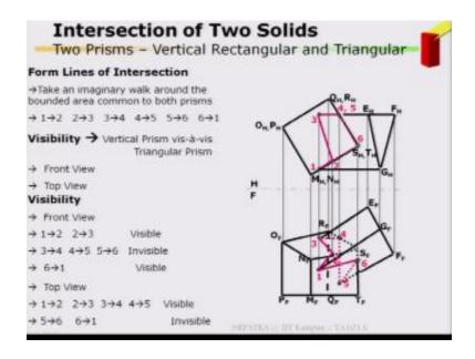
Once you get the interface surface I got the interface surface. Now you have to find it out the visibility, visibility means which is inside, which is outside. Which piers first which does not pier. So same method the visibility, take the two views, front view and top view, you do this visibility and find it out where is your visible, where is your not visible. Here 1, 2, 3, 4, is visible, visibility.
