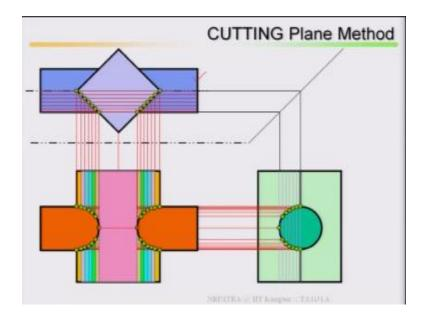
Now cutting plane method, cutting by plane method you take cutting plane, suppose this is one solid, this is another solid is going, there is a solid here one solid is going, take the cutting plane in between the intersection of the solids and I have taken one cutting plane here, then project it back how it cuts in your side view. Then you mark the point of intersection, from there you mark and you extend it to your front view, then mark your point of intersection in the front view.
