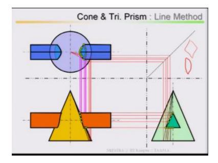
Now same intersection between cone and square prism by means of, intersection between cone and triangular prism. Earlier it was a square prism, intersection between cone and triangular prism example by means of line method, same way this cone has to be divided from there you project it back. Mark the points where is your intersections and from this projections you take out the cone and join it.
