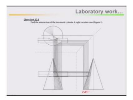
Top view front view and side view draw the side view same way find it out point of intersection draw the lines project it back then project it back, how in the top view interface looks like the surface. How in the front view it looks like. We have taken many number of points to get this smooth surface you name it, 1, 2, 3, 4, 5, 6, like this continue and you will get it.
