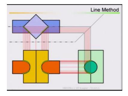
Now this is by means of line method, this is by means of line method, that means you take a line from your side view, project it back your top view, from top view you project it back front view, from here side view you project it back to front view, intersections and you mark it and draw, this is the surface, this is the surface at the interface, that means this solid and this solid at the intersections, interface, how your surface looks like? This is called by means of line method.
