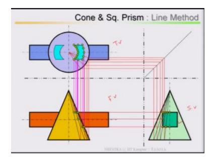
Then let us start with this, cone and square prism, cone and square prism by means of line method. Take your front view, take your top view, take your side view, in the side view mark the points, here, here, here, because inside this cone the square prism is there. This is your cone, inside the square prism is going. Now I divide this cone this half to this half into number of equal parts.
