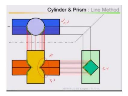
Draw the top view, this top view, draw the top view, draw the front view, this is your front view, this is your top view and draw the side view, draw the side view and from there with the side view take the lines, mark the points top and bottom, then project it back to your front view, project it back to your top view and this intersections points you mark it.
