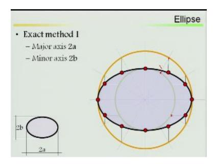
With this look at here, here, here, then point has been located, similarly you construct other part 1.2, 0.3 will be here, 0.4, 0.5, 6, 7, 8, then draw by smooth lines, draw by the smooth lines then it comes here ellipse, construction of ellipse.
