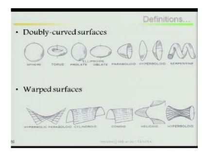
Doubly curved surfaces, warped surfaces.
