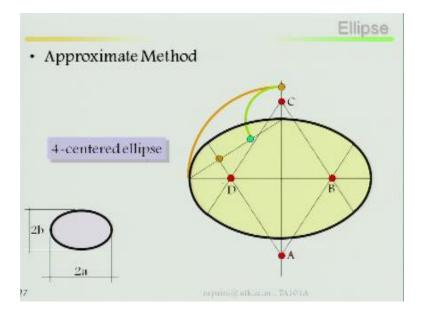
Then there is Approximate method that is called pore centre method. So consider major axis 2a this is a 2a that is a minor this is 2b, then join this major axis from here to here you join it, then considering these size radius draw an arc and mark the point extended part of your minor axis, this is your minor axis that means this is your b, this is your this part is your 2a and this is your b, considering this
