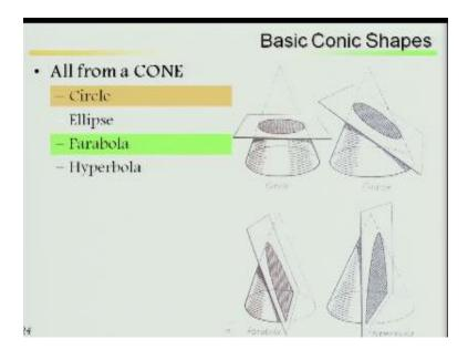
Then basic conic shapes all from a cone, hybrid is a circle, if I go with this if I make it, cut this cone here I can get a circle, if I certain inclination it will be resulted either ellipse, parabola or hyperbola.
