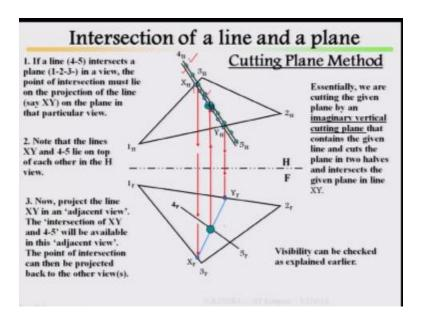
Point of intersection between (4, 5) and XY is the point of piercing point of the line inside the plane.
