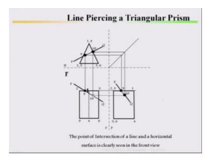
So if you look at here this is a triangular prism and line is piercing then you project it back, project it back, front view, top view, side view is given then find it out your piercing points. The point of intersection of a line and a horizontal surface is clearly seen in front, view take it, take it and look at it. I am just doing it very fast once you do the by means of cutting plane methods it will be very easy, one by one I am showing example.
