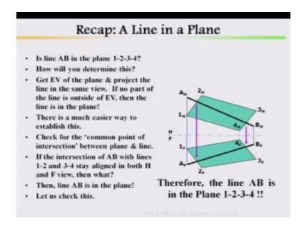
Then lines in a plane we have covered, this is what we have covered up to last class, lines in the plane, you can cross check with the opposite views and aligned it whether this lines in plane or not
