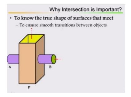
True shape of surface that meet to ensure smooth transition between the objects, suppose there are, one is solid object, another is solid object it is moving inside. What is that intersection? What is that intersection, what is the rear true surface at this junction?
