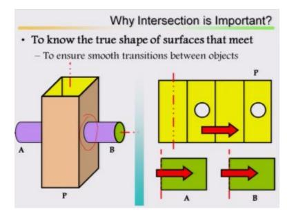
At the intersections, why intersection is important? Basically to know the true shape of surface that meet, true shape of the surface that meet to ensure smooth transition between the objects. I will stop it here, so next class I will explain more about this intersection of the solids. Thank you.
