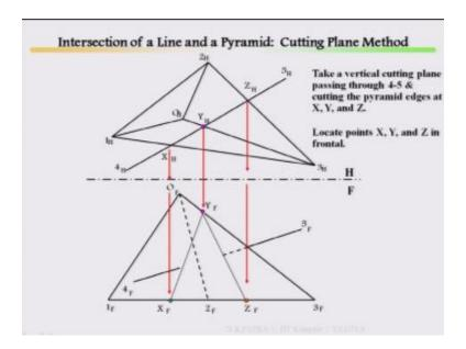
Now let us see intersection of a line and a pyramid by means of cutting plane, slightly, two are slightly difficult problem. This is your pyramid, and where is your line? There is a line and this is the line that means the intersection of a line and pyramid. Both lines has been shown in H view as well as frontal view. Now consider it, then next step take a vertical cutting plane passing through 4 and 5. So cutting the pyramid edges at x, y and z.
