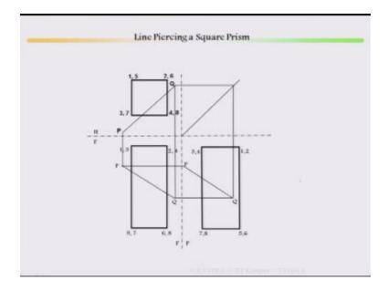
The next is your line piercing a square prism, three views has been given top, front, and side. The line is piercing in the top, line is piercing in the side, line is piercing in the profile view.
