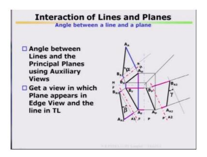
Now interaction of lines and plane, angle between a line and plane, angle between line and principle plane using auxiliary view how to get angle between a line and plane, you can do it by means of a auxiliary view as I said or by means of a edge view where the line will be taken as a true length, if you look at here
