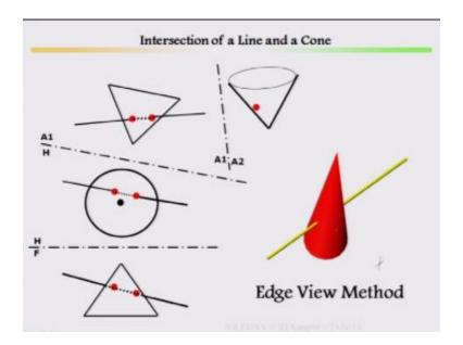
This is what I have said by means of edge view, by means of edge view there are two example one is your by means of cutting plane we have solved, now by means of edge view, edge view has been one auxiliary plane, edge view will come then from there you take the then line become line, then plane then where it is cutting, then you project it back, then you will get point of intersections. I am going slightly faster because it required for you to practice.
