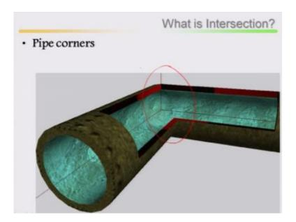
Then come to the second example, pipe corners, actually in practical utility where the drawing is required few cases I am showing, I have already explained lines, lines, line plane, line cylinder few examples. Now if you look at two pipes, two pipes corners, one pipe is going here other pipe is coming here at the corner how it, how it looks, at the corner how it looks this is called your intersection.
