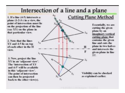
Now look at here, intersection between line and plane cutting plane methods. If a line, look at here, if a line (4, 5) this your line(4, 5) intersect the plane 1, 2, 3 in a view the point of intersection must be lie on the projection of the line say XY, say XY on the plane in that particular view. I have taken XY, note that the line x, y and (4, 5) lie on top of each other, in the H view.
