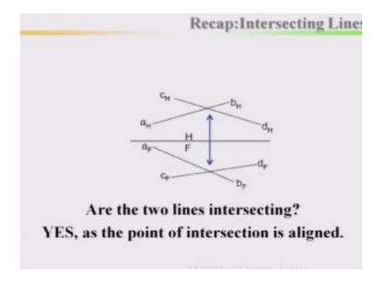
This is what we have covered, are these two lines are intersecting yes, as the point of intersection is aligned in the both the views
