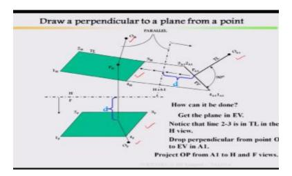
Been traced back, this is your point of intersection, then similarly it has been traced back to your opposite view that means your frontal view this distance d, remember once I am taking distance from here to here that means this is the distance in your opposite view
