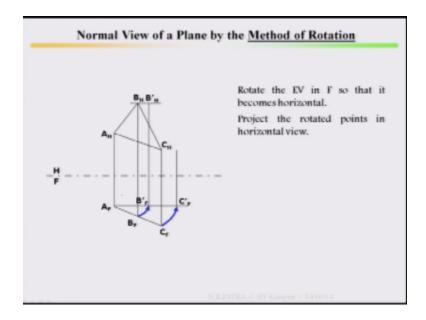
Then come to the method of rotations, this is a plane ABC, rotate the edge view in front so that it become horizontal. So rotate the edge view in front so that it become horizontal, this is your edge view it has been rotated so it become horizontal. So then ABC, ABC in frontal view has been rotated parallel to your hinge line, parallel to your hinge line. So this will be AF, BF and CF parallel to your hinge line.
