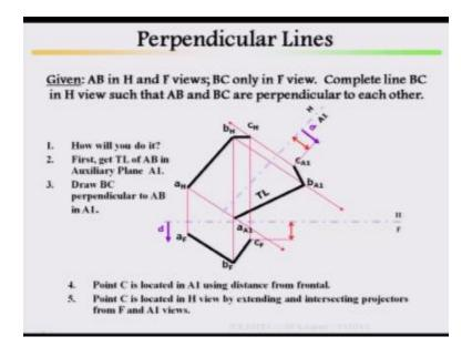
Given AB in horizontal as well as frontal view then BC only in front view, this BC is not given in the top view compete line BC in horizontal view, how will you do it? First get the true length of AB in auxiliary plane A1, draw it, measure the distance then find it out true length of the line AB then draw BC perpendicular to AB in auxiliary A1, right?
