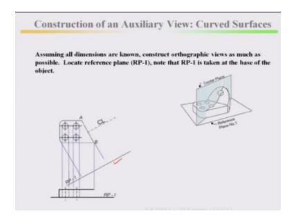
Assuming all dimensions are known construct orthographic view as much as possible, this orthographic view as much as possible. Locate reference plane RP-1 this is the reference plane has been made it here, note that RP-1 is taken at the base of the object.
