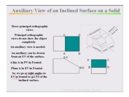
Draw principal orthographic views top, front and side, principal orthographic views do not show the object completely. An auxiliary view is needed. An auxiliary can be drawn from an edge view of the surface. A line is in point view in frontal. Plane is in edge view in frontal, the moment you go for auxiliary then a line will be a point and plane in edge view in frontal. So you go at right angle to edge view in frontal to get true shape of the inclined surface.
