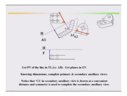
Take it, now take the point view, get point view of the line in true length that is AB, get the plane in EV, it is view then knowing dimensions complete primary and secondary auxiliary views this is the procedure.
