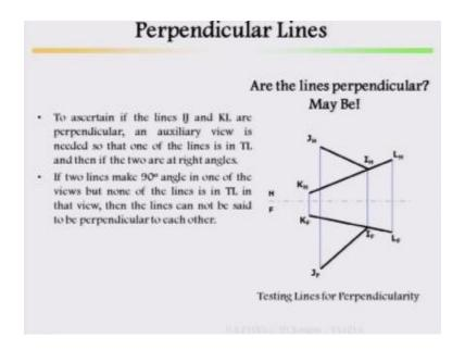
Look at here, perpendicular lines testing lines for perpendicular, perpendicularity whether the lines are perpendicular or not, draw the lines horizontal, frontal view draw it, are these lines perpendicular? May be, to ascertain if the lines IJ, KL are perpendicular an auxiliary view is needed so that one of the line is in true length, then if the two are right angles.
