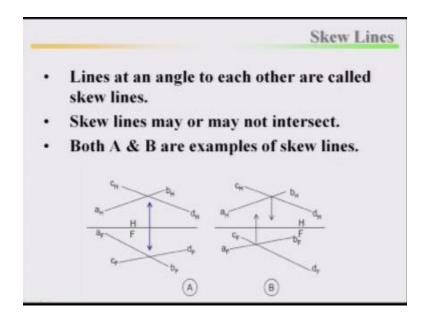
Angle to each other are called skew lines, skew lines may or may not intersect, remember here skew lines may or may not intersect, both A and B are examples of skew lines.
