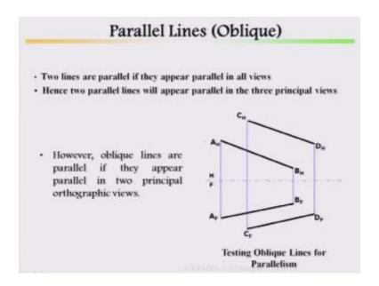
Parallel lines oblique two lines are parallel if they appear parallel in all views, hence two parallel lines will appear parallel in three principle views, testing oblique lines for parallelism, take it look at here, both this views top and front it is parallel, however oblique lines are parallel, if they appear parallel in two principle orthographic views.
