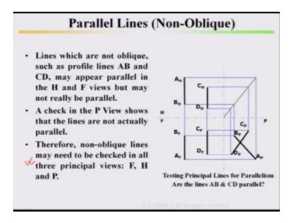
Then look at here, in this case parallel lines non oblique, see lines which are not oblique such as profile lines AB and CD may appear parallel in horizontal and frontal view but may not really be parallel, here lines appear parallel in top view and front view it is not necessarily that it is going to be parallel in profile view.
