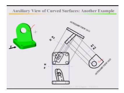
Front and top view you cannot locate the curved surface pictures, rather you go for, you go for auxiliary view 1 and auxiliary view 2, from there project it back to top view, project it back to front view then you can locate respective views of the curved surface
