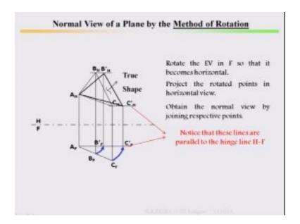
Then mark this points and join these and take it, because with respect to A it has been rotated edge view. So that means A is stationary, so your ABC, ABC it is your true shape of the plane. These lines are parallel to your hinge line of horizontal in frontal plane.
