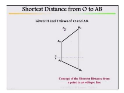
H and F view of O and AB, concept of shortest distance from a point to an oblique line this is your oblique line, this is your oblique line, then there is a point, how do you know that? In the space this point and this line will be somewhere else, how do say that it is the shortest distance? That means this line has to be converted to an true length, then bring back this point to that plane then draw perpendicular. So that you can say that this is your shortest distance.
