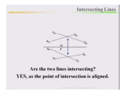
Here you see top view, front view it is aligned that means what we can say, are these two lines intersecting? Yes, as the two point of intersection is aligned.
