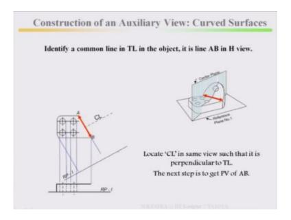
Then identify common line in true length in the object, identify common line in the true length in the object, so this is a common line, locate CL in the same view such that it is perpendicular to your true length, it is perpendicular to your true length, the next step is to get point view of AB
