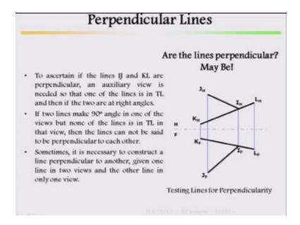
Sometimes it is necessary to construct a line perpendicular to another given one line in two views and the other line in only one view, these are the kind of say you can check whether lines are perpendicular or not.
