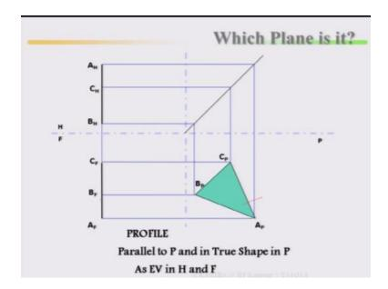
Means this part is your true shape, this is your profile, then parallel to profile it is in true shape in profile plane and as an edge view in frontal as well as in horizontal plane
