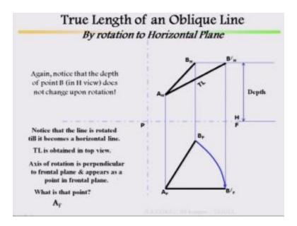
And rotation with respect to horizontal plane and the top view, rotation to horizontal plane, how to get the true length of a line by means of rotation.
