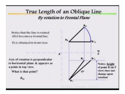
And the rotation with respect to frontal plane, how it has been rotated.
