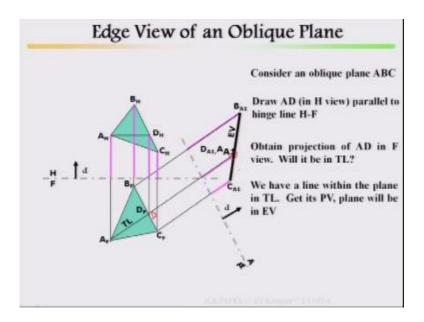
Now look at this edge view of an oblique plane, oblique plane in horizontal plane AH, BH, CH oblique plane in frontal plane AF, BF and CF, draw AD in horizontal view draw AD mark it, I just create a line parallel to the hinge line, in your horizontal view, either way you can do it, you can create a line CD parallel your hinge line in the front view I create a line AD which is parallel to your hinge line, then after projection of AD in front view.
