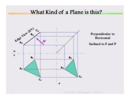
Then second edge view, edge view lying where, edge view is lying in your horizontal plane, that means this is perpendicular to your horizontal plane, inclined to frontal, inclined to frontal, inclined to profile.
