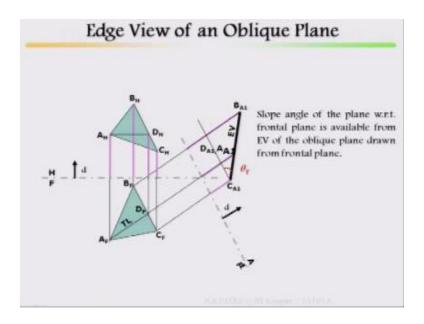
Look at here, if you look at here then this is your edge view then I draw a line parallel to hinge line. A line parallel to hinge line earlier example I am telling parallel to this hinge line then with respect to parallel to hinge line then this is your angle. This angle is your slope angle of the plane  $\theta_F$ . Slope angle of the plane with respect to frontal plane is available from the edge view of the oblique plane drawn from the frontal plane.
