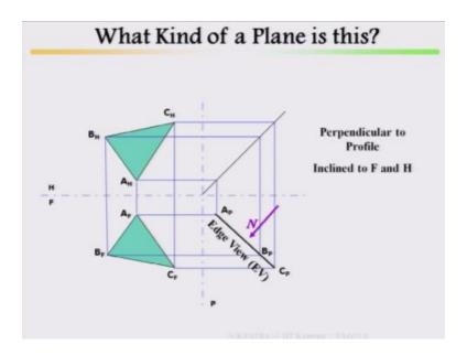
Similarly this is your edge view perpendicular to profile inclined to frontal and inclined to horizontal, perpendicular to profile, inclined to frontal and horizontal.
