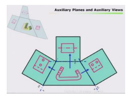
In this case, front, top, right hand side view, left hand side view. Now draw the hinge line, horizontal plane, horizontal plane top view will be there, frontal plane front view will be there, now look at here.
