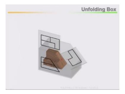
Then with respect to unfolding this box, how is your auxiliary plane looks like if you unfold it front view, top view and cut it, so this is your line of sight where it is perpendicular, so this will be coming to your auxiliary plane or auxiliary view.
