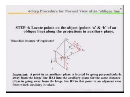
Now step 4, locate this, locate points on the object along the projection in auxiliary plane. So particularly if this is your auxiliary plane, then this distance as I said earlier this distance and this distance will be distance of the opposite view, that means this is your front view from your hinge line, that means this distance equal to your this distance and this distance equal to your this distance.
