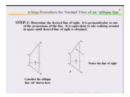
So first you determine your desired line of sight and it is perpendicular to one of your projection lines means desired line of sight whether which line you are going to do it then find it out desired line of sight. Then it is equivalent to one walking around this space until desired line of sight is obtained.
