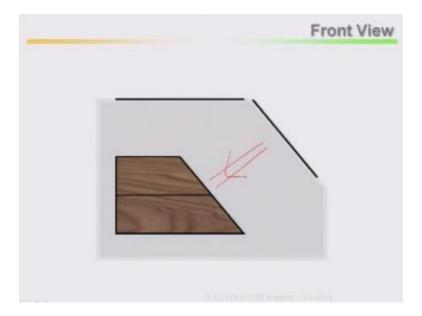
Now look at here, front view with respect to front view where is your auxiliary box? This is your front view and with this, this is your line of sight, this is perpendicular, this is your auxiliary line or auxiliary plane.
