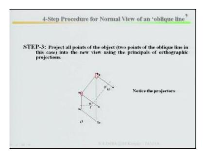
Now step 3 project all points of the object in a line, what are the points, 2 points of the oblique line in this case, into the new view 2 points of the oblique line in this case into the new view using principal of orthographic projections. Let us look at here, this is your auxiliary plane so from here I project it back, B point has been projected back, it has been projected back, notice the projectors, you notice this projectors.
