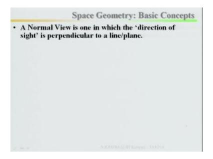
A normal view is one in which direction of sight is perpendicular to a line, this is a line I am looking it. A normal view is one in which direction of sight, my direction of the sight is perpendicular to a line or plane, my direction of sight is perpendicular here to a line and plane.
