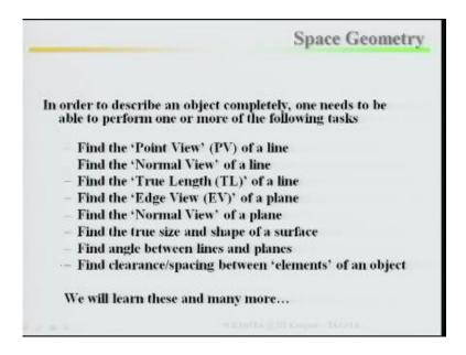
In order to describe an object completely look at this, one need to able to perform one or more of the following tasks, one or more of the following tasks. Find the point view, find the point view of a line, find the normal view of a line, find the true length of a line, find the edge view of a plane, find the normal view of a plane, find the true size and shape of a structure, a structure may be of any size any, any shape.
