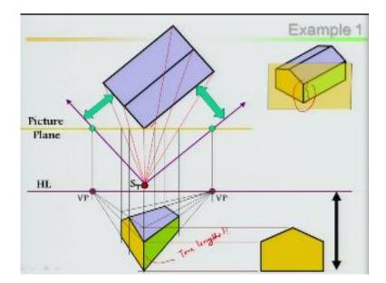
Maybe other part, so it touches your picture plane then  $S_P$  station point, from station point draw the parallel lines, parallel to your – this parallel to your left face, parallel to your right face. Then draw horizon line, then draw intercept from station point to your left face and right face. The parallel lines which intersect in the picture plane from there draw intercepts, then vanishing point 1 or vanishing point left, then vanishing point right.
