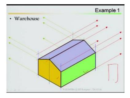
This can be done in both way, this warehouse, I can put it in isometric view so that I can see this side as well as this side or I can put this warehouse, just rotate it so that I can see it on one direction. So that means in this example there will be one vanishing point, as well as there will be two vanishing point. So in this case it will be a two vanishing point to take the clear pictures of both the sides along X and Y in isometric as well as Z. So that is why it has been rotated.
