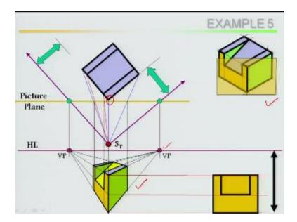
Then go to another example look at this, this is not a bread slice sorry, example 5 take the top view this is your isometric view, in the top view this isometric has been put it and this has been touch in your picture plane. Once this touch means this length will be in your true length, then locate your station point and locate your vanishing point left as well as vanishing point right, then take the side view, take the front view.
