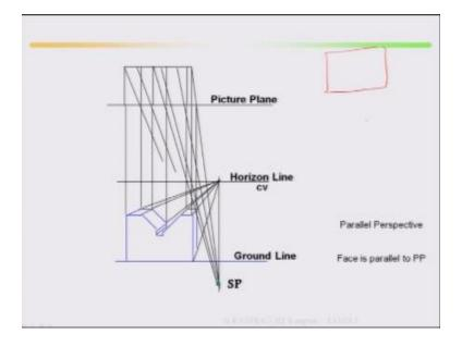
Now ground line, horizon line CV, picture plane, and station point.
