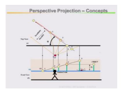
Ground line, front view, horizon line, horizon line is your coming eye ray then object and elevation you take it, station point and top view mark it and find it out where is your object starts, your object starts from here and it moves in this directions to infinity. So this is the big, so from here station point to object view look at there, then from there you project it back to your object line in the front view, this is in the front view mark it.
