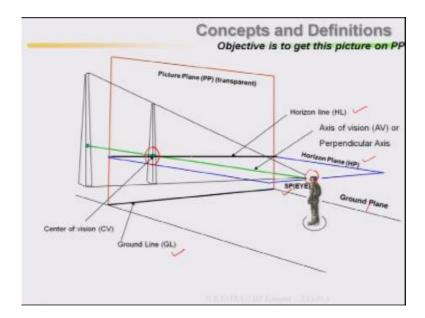
Ultimately the object has been projected back to picture plane, that means from station point to you have to look at the picture plane.
