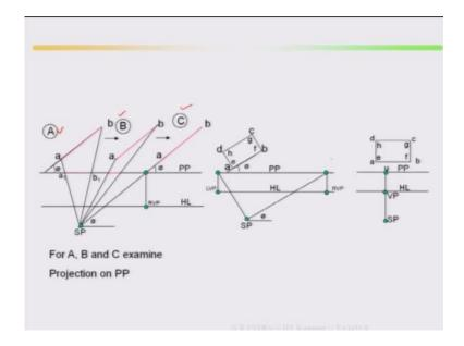
A,B,C, examine projections on picture plane A, this is you're A, B, then C, then again A, B, C, look at this is your station point horizontal line, horizon line, picture plane, station point, horizon line, picture plane, how it is moving A, B, C? Before I come to this.
