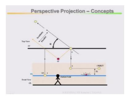
Now point four, suppose in the picture plane draw join from station point to point four, and once this because top view will be somewhere else here. So find it out the where the view point is there, then from there draw the line, perpendicular line where it cut your object, parallel to this mark this point, point four. Similarly from station point to mark objects from point, here is your tip view it is going, then infinity.
