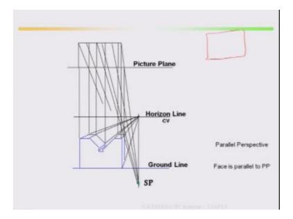
First let us consider parallel perspective, face is parallel to picture plane, in parallel perspective face this object face, this is the face this face is parallel to picture plane, face is parallel to picture plane and there is a horizon line CV, ground line, and station point.
