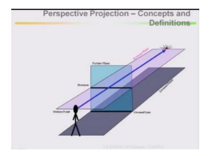
Now concept and definitions, these are all to understand what do you mean by your perspective view. Now let us — this is a ground plane, ground means where I am standing. If I am standing here this I can define as a ground plane, here this is your station point, station point means where you are standing and looking at the object that has been called station point. This is your ground line, then this is your picture plane, this is your picture plane.
