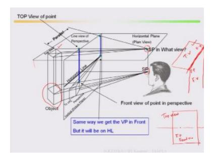
Let me go to the 3D view. All we are doing 2D view, you can imagine in a drawing sheet generally what happen in a drawing sheet we divide into two parts, we say these are my hinge line and this will be my top view or top view plane or this will be, in this case I can draw or this will be my frontal plane you can write it FP where you can draw front view, I can draw this in this way.
