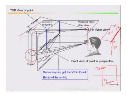
Now if I come here top view, station point so if I rotate it back this station point will be somewhere else because this is my hinge line with respect to from here to picture plane to some distance station point, again I have to rotate it back then your front view will be somewhere else. So this is the basic principles.
