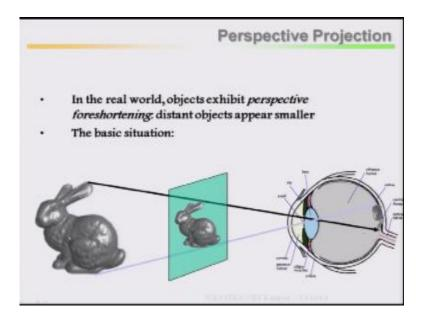
If I take a picture plane in between object and the eye, if I take a picture plane, so it is in between the actual object and what I visualize in between it is a medium size.
