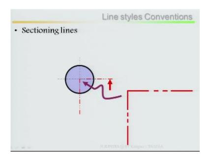
Then sectioning lines look at this sectioning lines how it looks your sectioning lines, if I say one half has been sectioning line has to be plot how your sectioning lines, one line two dash then continuing as second line, one line two dash continuing second line, then both the lines to join there should not be any gap.
