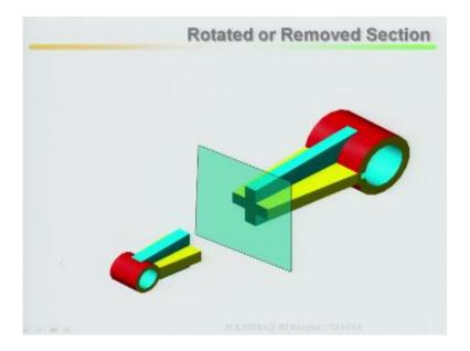
Then rotated in removed section.
