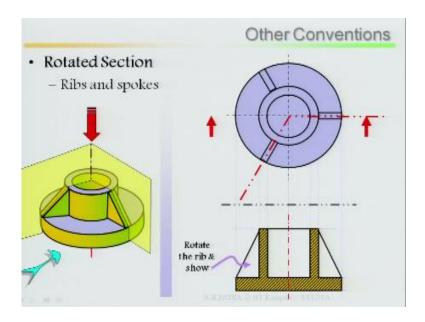
And spokes, now we can rotate the ribs I can rotate the ribs, rotated sections if there is a rib of this planes this planes and this place, here it is your cemented line, so you can rotated back bring back your center line of you sectioning exactly it has been done it has been rotated back, it has been though it has been rotated back. So you can show it symmetry, so that people can understand it has been rotated back.
