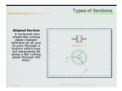
Then align sections, align sections if there are cases where your holes are not symmetry and at the same times maybe holes are different holes, then you can put align sections. So that you can, so pictures inside this hole.
