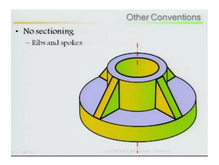
No sectioning ribs and spokes particularly ribs and spokes these are the ribs.
