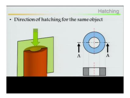
Now direction of hatching for the same object if I cut it then I have taken out the front and looking at from the front side front view, how your hatching is? It should be in the direction of the hatching for the same object section at AA.
