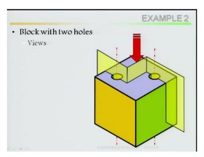
Then block with two holes look at the block there is a block two holes opposition to each other example two, now what is your view? What kind of sectioning I want to do It? These are not symmetry rather this is diametrically opposite. So align sectioning in this case align sectioning has to be done. Now a plane has been taken here passing through the hole then with your 90 degree and taken center line of the hole second plane is going. That means it is align.
