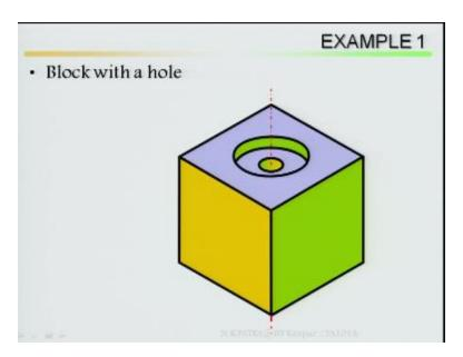
Block with a hole example 1 there is a block and with a hole, imagine this block there is a block and if I look at this isometric view this is a block there is a hole at the top this hole is continuing upto certain distance then after that there is a inner hole also there that means this hole is not throughout.
