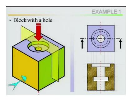
Now you are looking this object from this side, take this object from the top view you can even put it at the top view, then front view you draw, how it looks? Then take a cutting plane, cutting plane in such a way that you can see the inside features or inside view I am taking a cutting plane in the symmetry with a vertical axis. So that it pass at the center of the hole. So that it is symmetry.
