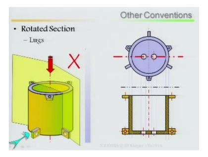
You cannot do it by means offset sectioning or by means of align sectioning, rather this is wrong.
