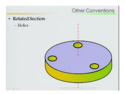
Rotated section holes suppose there are three holes not align with each other, then always you can rotate.
