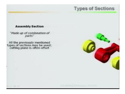
That means it is the combination of different parts example these are the different parts and it has been assembled first then sectioning has been made.
