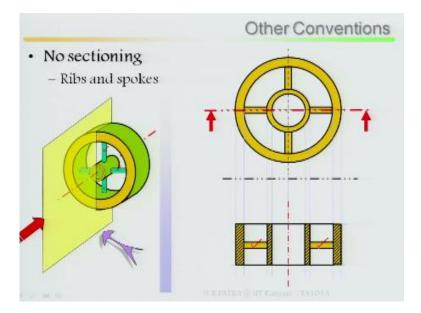
Same thing look at the inside of feature of the ribs, no sectioning, no sectioning means, no hatching am not doing any hatching here, because these are my rib part, these are the materials connected by the rib here, here, here but this is the material so here it is no sectioning that means no hatching.
