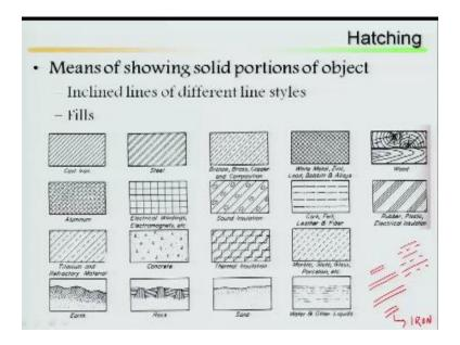
Now come to the hatching, for different materials there are different types of hatchings once you put that hatching during sectioning that means it shows that, that material is made up of what kind of material, if you looked at here custodian how is your hatching has been done and still particularly still two parallel lines then there is a gap still is two parallel lines then there is a gap again two parallel lines parallel to earlier two parallel lines two parallel lines.
