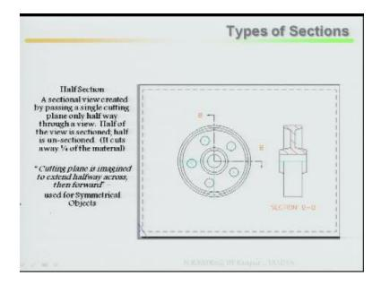
Second one is your half section, only half of the when there is a symmetry both the sides only half of the sectioning can be done.
