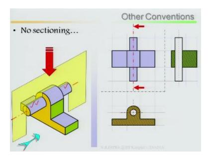
Look at your shaft, I cut it at the middle that means half, full sectioning has been done, then the material has been taken out. How it looks your shaft that means no sectioning has been done particularly in shaft have you mark it, this is your shaft this part is your shaft it is going throughout, this is a material, and this material has been put it. But the moment you cut it the shaft has not been section, cut it in this way, how it looks.
