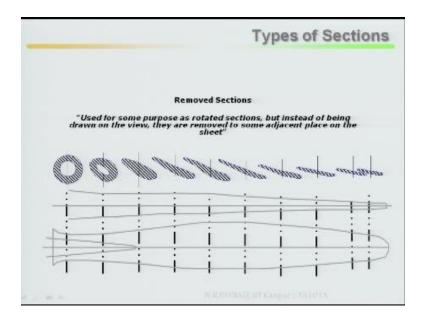
As I vary from section to sections the removed section looks like this, it is changing from one plane to other plane.
