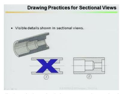
Then invisible details shown in the sectional view once you take a section, inside the sectional view visible details example 1 a and b. So example a is in correct, particularly striking at section here for a it is incorrect but section taking at section the sectional view in b it is correct.
