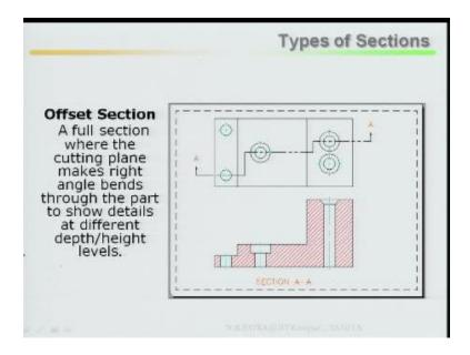
If there are full section where the cutting plane makes right angle bend through the part 2. So the details are different depth and height to so the parts in different depth as well as in height in that case you need to have to have your offset section.
