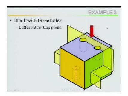
Block with three holes different cutting planes.
