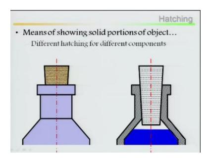
Meaning of showing solid person of a object different hatching for different components, we have started now hatchings.
