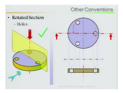
If you look at here this holes in a plate three holes then take a section draw the top view, draw the sectional line where you are going to do this sectioning and which view, which side you are going to view. I want to do the sectioning cutting plane putting here and taken out the entire solid up my front ways and looking at the, from front view, then what you are supposed to do? You rotate this hole back to here or maybe you can rotated it back to here, put it in the align in the center line.
