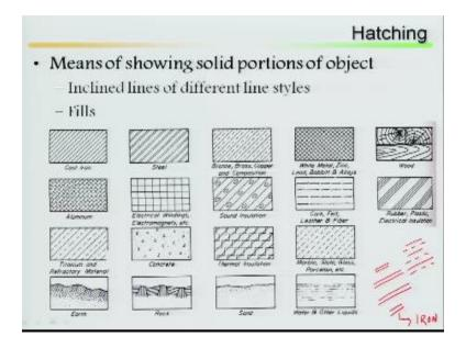
First one is your means of solid person of the objects solid person of the objects what are the different hatching lines?
