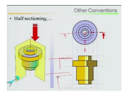
How it looks your half sectioning, the moment I say it is full sectioning that means, from here to here the moment I say it is full sectioning from here to here, the cutting plane should be throughout and I will take out half and look at it. Why it is half sectioning? This is axis symmetric problem that means throughout if I take one quarter, half of the sectioning whatever I am going to see it will be throughout set.
