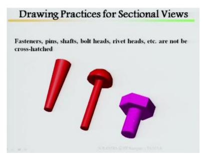
Fasteners, pins, shafts, bolt heads, rivet heads are not the or, are not suppose to be hatched. Fasteners, pins you put the pins inside, then bolt heads these are not suppose to be hatched, like screw these are not suppose to be hatched. So I will stop it here, so next class I will start assembly sectioning with typical 2, 3 example so that it will be very easy for understanding. Thank you.
