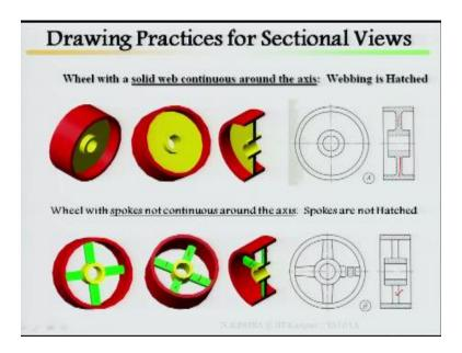
Start with this typical and find of a you can say that this is assembly, if you remember well different types of sectioning, full sectioning, half sectioning offset align rotated removed and other one is your assemble section. Now we are coming to assemble section wheel with a solid web continuous around the axis, there is a wheel with a solid web continuous around the axis. Webbing is hatched in this case webbing is hatched looked at here, how it looks then how it looks, when I cut it.
