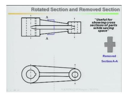
Middle part, how it looks? Then it has been rotated to see both the sides how it looks both front as well as rear, then this rotated section has been removed and placed separately.
