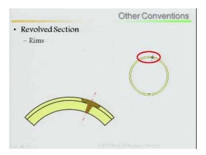
Rims look at the rim, revolved section rim there is a rim here, how the sectioning has been done in the rim not the entire rim, the revolved section how it has been done one part.
