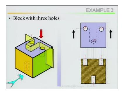
Look at your top view this is the hole, now plane has been passed through first hole align back then it has been passed through your hidden hole then again align back then it has been passed through your second hole. So that once I take it out I can once I do the plane cutting plane here if I take out here and looking from the front that means this half I can see this half I can see, how it looks?
