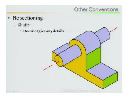
Now no sectioning, there are other certain conventions other conventions no sectioning shaft particularly shaft remember, number one shaft, so shaft does not give any details, so that means if there is a shaft in case of shaft no sectioning should be done.
