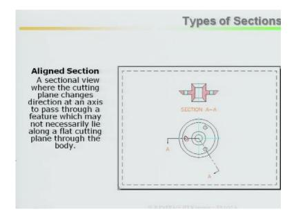
Our direction at an axes to pass through it picture which may not necessarily lie along a flat cutting plane through the body aligned sections you see what happens if you looked at here if am putting is sectional plane here this part lying in this body but if you looked at her if I am cutting this part is missing this part is missing so I take it and align where the other part is there.
