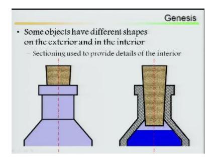
If I cut it longitudinally, if I cut it longitudinally then I am able to know if there is a cork how far it has gone inside, what is its depth inside this bottle. So outside it doesn't reflect anything, but if I cut it at longitudinally looked at their – the cork has been penetrated here or pushed inside up to this depth here. So this is what you are going to show in sectional view.
