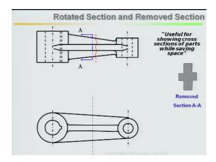
This is almost aerospace mechanical civil engineering also this rotated sections and remove sections are very much useful for showing cross section of parts while saving space while saving space.
