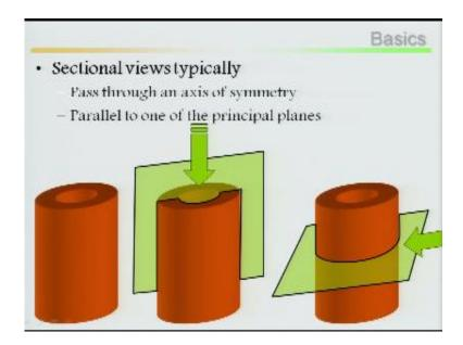
Then this is at your top front view that was longitudinally you cut it, make it longitudinally two parts first one, so that you can see in front face what is inside. Then at the top you can cut it, top you can cut it at the top or maybe at the middle, I can cut at the middle. So parallel to one of the principal planes.
