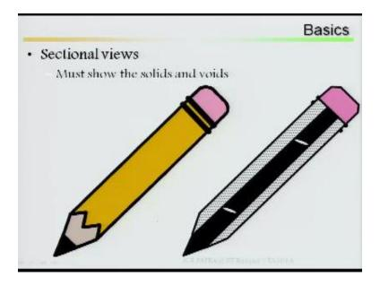
Sectional view you should show this solids and voids, simple pencil if you take it, simple pencil. Pencil is made of what? Simple example, solid covered by wooden lead covered by the wooden. So wooden is a different material, lead is a different material lead has been covered by this wooden and there is cap backside sometimes pencil cap is there, there is a simple pencil this is a wooden and here I can see the lead whether this lead is throughout or not I do not know.
