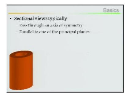
Sectional views typically pass through an axis of symmetry as far as possible pass through an axis of symmetry parallel to one of the principal planes. I have said in the beginning parallel to one of the principal planes.
