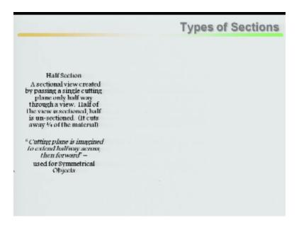
Use for symmetrical objects, particularly why half of the section if you do, one half whatever the material is there, second half or the other half same material will be there, if it symmetry not necessarily so the entire sectioning rather used half of the sectioning.
