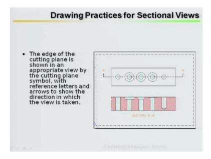
How it looks the edge of the cutting plane is shown in an appropriate view by the cutting plane symbol with references letters and arrows to show the direction in which the view is same thing as I said.
