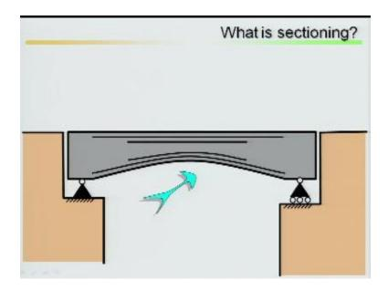
Let us start with simple example a bridge is there, then a beam or rider is there with a roller as well as support, roller support as well as a hind support.
