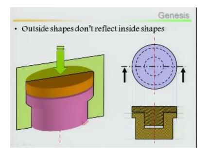
Let us cut it longitudinally along the arrow make the half, do the sectioning. Now once do the sectioning you can imagine this is not the thickness throughout, outside cap is not thickness throughout there is a thickness, then there is a cover narrow down then it has been pushed inside. Again in this case there is a gap at the top, so it is a air tight or maybe tighten from the top it has been pushed. So it reflects inside shape of the object.
