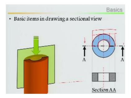
Basic items in drawing a sectional view, what does it mean? I cut it longitudinally then want to show what is the basic material, how the material has been made. This material is throughout solid or hollow or some part is hollow again throughout the solid. Unless if you are not cutting it and looking it inside you cannot define it. Sectional view at AA, in this case what happened, longitudinally it had been cut from the top view.
