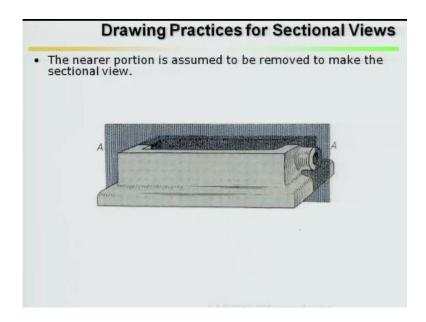
The nearer person is assumed to be removed to make this sectional view. If I am cutting this nearer personal assumed to be removed I am cutting this plane and this part as been removed.
