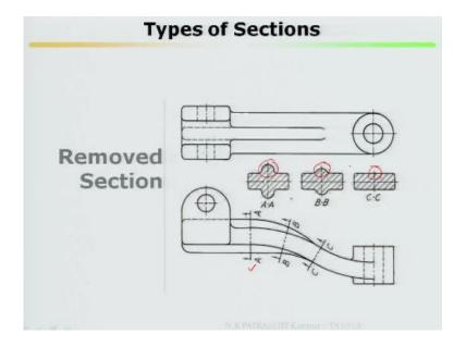
one more example removed sections look at this object top and front view and it has been made at A-A, B-B, and C-C how section it look like at A-A this sectioning as been done they can and sectioning sectional view has been drawn here B-B sectional view has been drawn C-C sectional view has been drawn looked at it how it is varying from section A-A, B-B and C-C in C-C while reaching from A-A to C-C this part is slowly, slowly managed.
