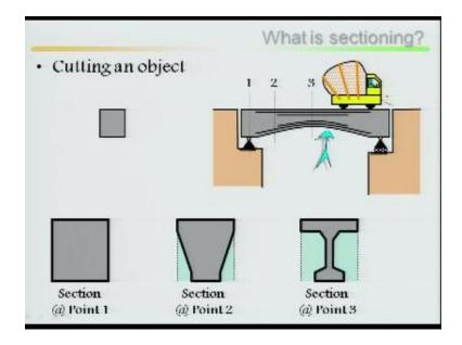
If I take it cutting an object this is your object, this beam I want to cut this object at different sections. Outside it does not look good, if I cut it look at here section 11, at these section, section 11 how it looks. The section 11 section is simple, rectangle or square section 11. Come to this section 2 at point 2, I can write it 11 at point 2 I cut it, look at there, section 22, look at this how it looks section 22.
