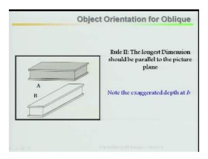
Rule 2, longest dimension should be parallel to the picture plane. So these are the two rules you have to follow in case of oblique drawing.
