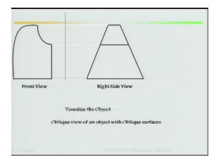
This is your oblique parallel projections, this is your front view slightly complicated case one example, right side view, visualize the object, oblique view upon object with oblique surface, this is a typical case oblique view upon object with oblique surface.
