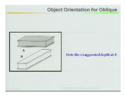
Number 2, note the exaggerated depth at b. This is your B this is your A, in case of A and B this is coming as a width, in case of B the depth direction is long, the depth direction is long.
