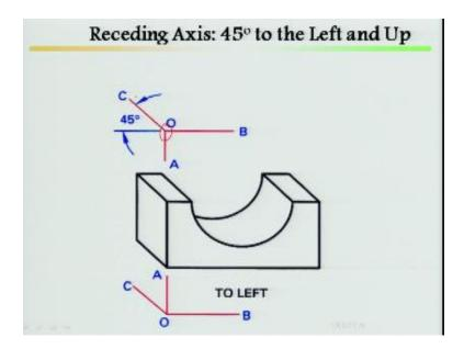
Receding axis 45° to the left and up. I am sitting here if I sit 45° to the left and up in depth directions that means here 45° to the left, this is the left. So here 45° to the left and up, up means with the normal axis it is up.
