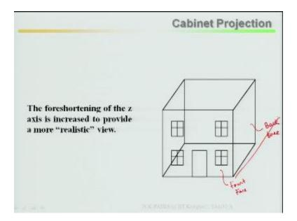
In depth direction suppose depth direction is large, suppose in this case this side is your – this is your front face, this is your rear or back face you can say back face, suppose in depth directions it is larger. In the back face there are certain features, so to show it and bring it closer so that you can visualize. So that is the object behind this cabinet projection.
