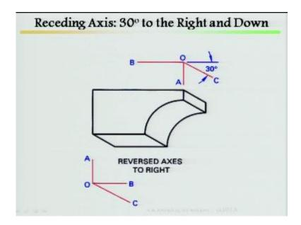
30° to the right and down, remember this notice hence in the exam this will be given the notice 30° to the right and down, 30° to the right from here 30° to the right, here in this direction right and down, down means with the normal axis it is down to your normal axis. This way it will be given, kind of the question will be asked. Draw a cabinet or cavalier view, where you are in a depth direction 30° to the right and down. That means it will be down and 30° towards your left.
