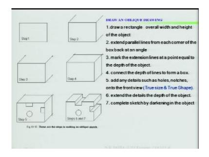
Last class we have finished basic introduction to oblique drawings. So we have covered one examples and steps. So just for a repeat step 1, draw a rectangular a rectangle overall width and height of the object step 1, because the front face is giving your true shape. Extend parallel lines from each corner of the back box at an angle, mark extension lines at a point equal to depth of the object.
