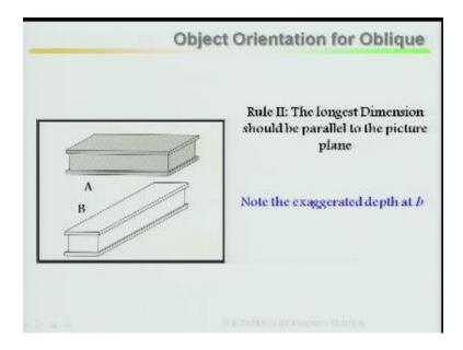
In that case rule 2, the longest dimension should be parallel to the picture plane. Longest dimension should be parallel to the picture plane. In this case this is your shortest dimension; this is your longest dimensions.
