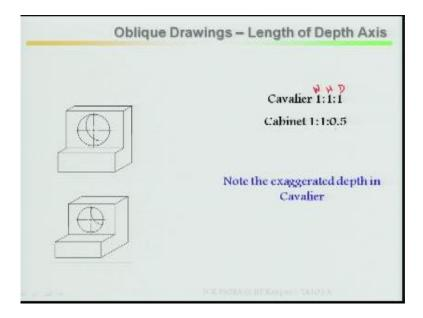
Oblique drawings length of z axis cavalier remember 1:1:1 that means it is completely true shape, true shape and I am not saying about true shape completely same length, same dimensions front face is your true shape. So 1:1:1 that means width, height and depth 1:1:1. Cabinet 1:1:0.5 remember this is your width, this is your height, this is your depth. So here cabinet 1:1:1 then 0.5, 0.5 this is in your depth directions.
