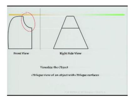
Look at this object visualize, front view and right side view, front view and right side view visualize this object. This is your oblique surface, this is your oblique surface then it is a simple case of oblique view upon object with oblique surface, front view is given the right side view is given.
