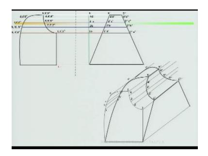
Once you finish it up you are finished curved surface inside, inside feature of your curved surface, because prime objective of this oblique projection is, if there is a curved feature that has to be shown clearly in case of oblique projections. So then this is what how your front size this is your front then this is your rear side then which part I can see it, exactly which part I can see it.
