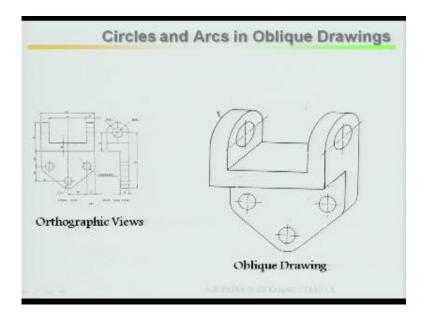
Circles and arcs in oblique drawings, orthographic views then oblique drawing, how it looks for visual eye sense. This is your orthographic view, front view as well as side view, then oblique drawing how it looks.
