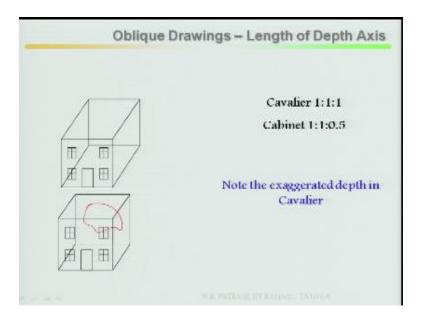
Look at the two drawings length of depth axis one drawing very simple picture a building, one drawing in the depth axis, it is a large dimensions. So if you bring back, if you bring back to the front the back side you can very easily visualize what is there in back side, so that is the reason this cabinet view are oblique drawing is there, but the objective of this oblique drawing particularly our cavalier as well as cabinet.
