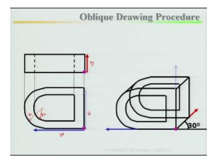
One this example I have finished, this two examples I have finished take your reference line, reference point then width mark your width, mark your depth, then mark your height. Then in depth directions make an angle with 30° this is your depth directions, this is your depth direction, this is your width, this is your width, this is your height, this is your depth directions. Then as front view it is in true shape.
