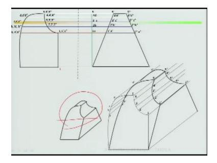
Then once again I am explaining take a reference point reference line then mark your oblique surface different sections, mark the points. Then once your front face or front view has been given in oblique projections front view is your true shapes. So finish your front face or front view, because this is your true shape. Then go to your depth directions then mark the same way, the way the points are been – or sectioning has been marked and points has been located.
