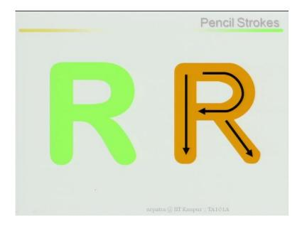
Then R, stroke one, stroke two, and stroke three, if you look at your R how do I write the R?
