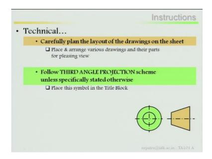
So technical, before coming to drawing class carefully plan the layout, once you are in drawing class carefully plan your layout of the drawing on the seat, place and arrange various drawings and their parts, generally in drawings we follow third angle projections scheme unless otherwise it is not specified, later on I will explain what is.
