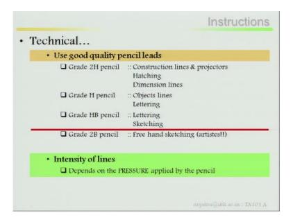
Then these are the pencils, grade 2 expenses as I said earlier, constructions lines and projectors, hatching dimensions lines, generally it has been done by means of your 2H pencils, then grade H pencils or H pencils particularly for objects lines, lettering, HB pencils lettering and sketching, grade 2B pencils generally free hand sketching or artistics, this is all about introductions of your engineering graphics or TA101 course.
