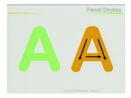
The A is looking like this, now the sequence is, this is my first stroke, second stroke, then this will be a third stroke
