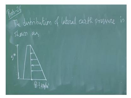
So, the distribution of lateral earth pressure is shown as so this is the wall okay the total height of the wall is say 5 m and your lateral earth pressure is shown here so that is 43.3 kN/m square at the base okay 43.3 kN/m square per meter run of the wall okay. So, therefore the first part is over the first part you have to find out the distribution of lateral earth pressure on the retaining wall. So, that already we have got it. Now the second part.
