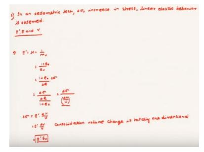
Now it is said that in an oedometric test for delta sigma v increase in stress a linear elastic behaviour is observed. So, it is clearly given that the linear elastic behaviour that means all the definitions that we said in the previous part are all valid. Now in this case you are asked to find out the relation between oedometric modulus E dash the Young's modulus E and nu. So, as I
