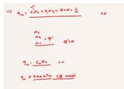
Now this has not been covered and this is a introduction to the foundation engineering so I will just cover a basic formula like the bearing capacity C into N c + q into N q + B gamma N gamma into half. Now here N c, N q, and gamma are basically, parameters that basically, are depending on N c, N q, and gamma are the parameters that depends on phi dash. So, this is where the phi dash comes into problem.
