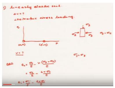
So, basically, the problem stated that a linearly elastic soil was present and you are supposed to find out the change in the volume that is delta v when subjected to isotropic stress loading. Now we also said that the isotropic stress loading is basically, in a pq space. An isotropic stress loading means this the sample is not subjected to any shear stress. That means basically, if the sample starts from a point at 0,0 then it will be at some point P dash 0 after an isotropic stress.
