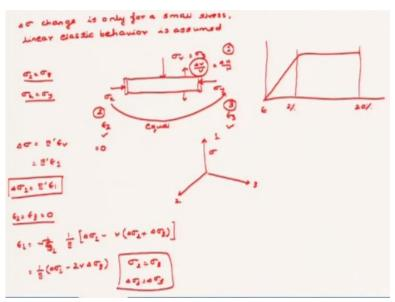
So, one thing you should remember that this delta sigma change is only for a small stress linear elastic behaviour is achieved. That is obvious because if you perform a if you perform a stress-strain test as well triaxial direct shear or oedometric you will see that this elastic range is very
