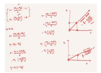
So, now from our definition p as you know is sigma 1 + sigma 3 by 2 while q is equal to sigma 1 - sigma 3 by 2. Now this is valid for a 2-dimension case. In 3D p can be defined as sigma 1 + sigma 2 + sigma 3 by 3 while q is equivalent to sigma 1 - sigma 3. Now generally these are termed as the s t ten sets. This is also defined by the name of s t while this is defined as the name of p q in that case.
