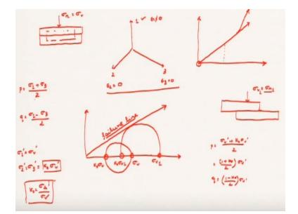
So, if you take into consideration the effect of consolidation then in that case it is different from an isotropic compression because in this case again if you consider the if you consider the effect of consolidation then you just apply the load here sigma n which is equal to sigma v and you apply the consolidation to occur. Now obviously you do not know what is the horizontal or what is the what are the horizontal stress.
