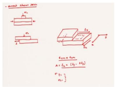
Now for the next part it is asked the stress path of a direct shear test. Now before you start before you start moving over the direct shear test let us discuss a bit about the direct shear test and how the stress path should be just like the consolidation test. So, as you know in case of a direct shear test there is a shear box that is again confined in this 2 directions and a load is applied from here. This is the normal load. This is the sigma n or the normal load.
