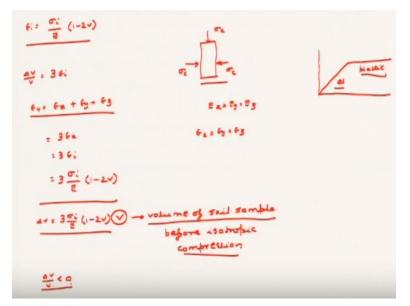
Now this can also be written as so epsilon i is equal to sigma i by E into 1 - 2 nu. The volume change as we all know is equivalent to 3 epsilon i. Now how did I get that? This is because the volumetric strain epsilon v is equivalent to the strain in x direction the strain in y direction and the strain in z direction. Now from the problem itself it is given that actually it is an isotropic stress loading.
