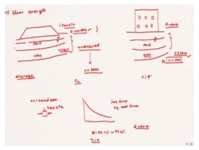
Now the next part that to move is basically, the shear strength and consolidation. Now these 2 parameters are going to tell you that whether your soil is going to support the given load or not. So, from the point of shear strength view from the point of shear strength what you have to do is
