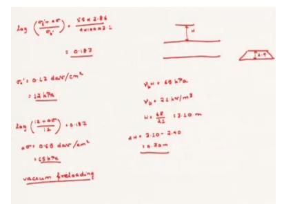
So just plug the values and you will get log of sigma 0 dash + del sigma by sigma 0 dash as 55 into 2.86 divide by 4 into 100 into 2.1. This is equivalent to 0.187. So, from here you already know what is the value of sigma 0 dash is because sigma 0 dash is basically the stress at the mid height of the clay layer. So, the stress at the mid height of the clay layer corresponds to a value of 0.1 0.50 0.12 da newton per centimeter square or basically 12 kPa.
