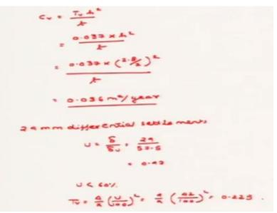
Now from T v we will calculate the coefficient of consolidation. So, T v into h square by t the formula for coefficient of degree of consolidation. So, T v as we all k now we have founded out
