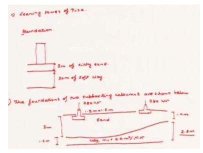
An example a very good example of the different settlement is as you all know is Leaning tower of Pisa. Now in this case when the when the end at the end of the 1178 when the structure was completed the tower began settling differently. The foundation in that case let us say this is the structure then this is 3 m of silty sand and this was the clay layer that was 30 m of soft clay. Now this 30 m of soft clay was the only reason why basically it caused the differential settlement.
