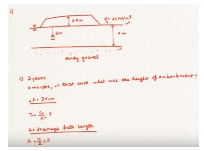
So, we are discussing here a problem on consolidation which basically stated that there was an embankment of height 4 m, height 2.4 m below a clay layer of 4 m. So, the figure was this height was given as 4 m this embankment height was given as 2.4 m the gamma of embankment was given was 21 kN/m cube. Basically, this is the gamma b or the bulk gamma.
