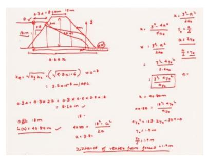
So, now this is the dam this is the earth dam. This is the z direction this dimension is obviously the vertical dimension is unaltered. So, this is obviously 18 m again. The height is 20 m again and the horizontal length I mean this length this length whatever it is has been multiplied by 0.6 into x whatever the dimension may be. This is what the this is what is the altered dimension.
