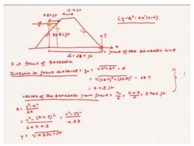
So, now our dam upstream level is known to us as well as you know from where basically the parabola is going to start. So, this distance is known to us. This distance is given as 9.84 feet. So, this is the starting point of our parabola. So, is where the parabola will start. Now we all know that F is focus of parabola and the point F lies exactly here. So, this is the focus of the phreatic line itself is a parabola.
