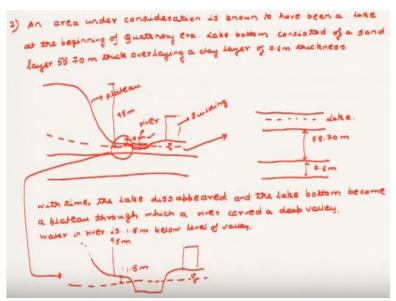
So, let us start with the problem. An area under consideration is known to have been a lake at the beginning of quaternary era. Lake bottom consisted of a sand layer 55.70 m thick overlaying a clay layer of 7.6 m thickness. Now let us see the diagram how does it look like. So, this is how it looks like and this is where the present water table is and a building is constructed here. So, this is let us say the lake bottom.
