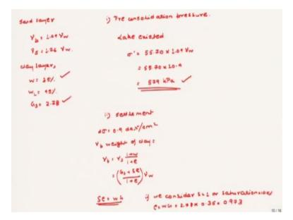
Now the first question that is asked is given the sand layer as gamma b as 1.04 gamma w gamma s as 1.76 gamma w clay layer as w as 35 percent W L that means the liquid limit as 45 percent and G s or the specific gravity of soil solids as 2.78. You are asked to find out the preconsolidation pressure first. Now how do you calculate the preconsolidation pressure because finding out the preconsolidation pressure is the first fact that requires nothing.
