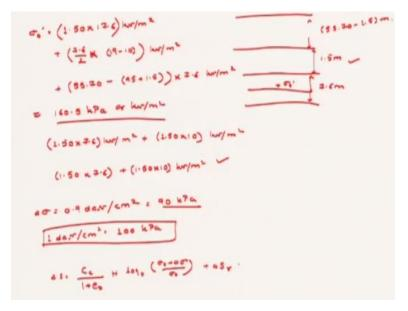
Now since the height of the capillary zone is 1.5 m so we will have sigma dot that means that the middle of the clay layer if you consider now the sand layer has a height of capillary zone of 1.5 m then 7.6 m you have to find the height at here that is the mid height what is the sigma 0 and above it this length is 55.70 - this 1.5 m. So, if you find it out then this is 1.50 into now what is the unit weight of sand at that point is 17.6 so 17.6 kN/m cube meter square this is for this layer.
