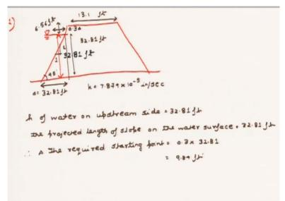
It says that a dam is given to us where basically the water at the upstream level is at a height of 32.81 feet and the water on the downstream level is at 0. So, basically now you have to you are not given the phreatic line and you have to draw the phreatic line through this earth dam. The other dimensions are given as the top of the dam is given as 13.12 feet and this height is given as 6.56 feet.
