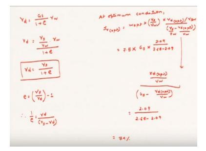
Now how do we get the expression gamma d is equal to gamma s by 1 + e this from the general relation that gamma d is equal to G by 1 + e so basically into gamma w. So, basically, we write that gamma d is equal to gamma s by gamma w into gamma w by 1 + e. So, gamma d is equal to gamma s by 1 + e. So, from here we obtain that e is equal to gamma s by gamma d - 1. So, we can also write 1 by e is equal to gamma d by gamma s - gamma d.
