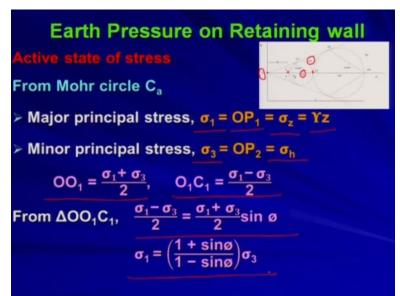
So, in case of active state of stress so from the Mohr circle C a as I told you in the active state of stress the major principle stress sigma 1 is equal to O into OP 1 okay so O is the origin okay and P 1 is this point. So, OP 1 is your sigma 1 which is nothing but your sigma z that is that means sigma v right sigma z and sigma v both are same so in the z direction that is why I have written sigma z to understand this thing more clearly.
