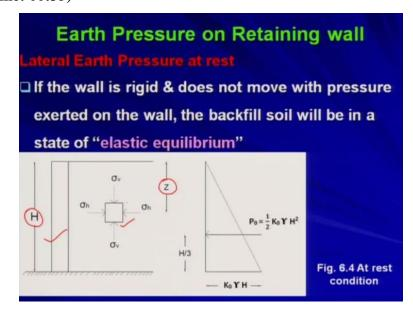
So, now in this lecture we will be talking about the elastic equilibrium and we will be trying to establish the relation or trying to establish the expression for earth pressure at rest and earth pressure at active and passive condition. So, if the wall is rigid and does not move with pressure exerted on the wall the backfill soil will be in state of elastic equilibrium.
