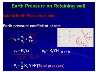
So, now first we are going to find out earth pressure at earth pressure coefficient at rest condition. So, earth pressure coefficient at rest condition is defined by K 0 which is nothing but sigma h by sigma v that is the definition of the earth pressure coefficient. Therefore, that is nothing but sigma h. Now what is sigma v that is nothing but gamma z am I right. So, if you know K 0 and if you know at what depth you are considering so therefore sigma v is known to you can find out sigma h.
