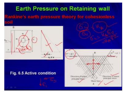
Now in case of active condition we are trying to obtain this kind of say or we are trying to develop this earth pressure coefficient or the relation between the vertical pressure and the horizontal pressure in case of active state. Now and that was proposed by Rankine's okay so therefore that is why it is known as Rankine's earth pressure theory for cohesionless soil. So, first we are considering the cohesionless soil that means c is 0 okay.
