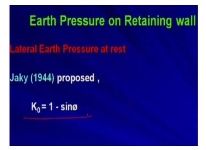
Now Jaky in 1944 he proposed that K 0 can be taken as 1 - sin phi where phi is the angle of internal friction of the soil and it has been found that this value of K 0 gives very good or reasonable result in the soil mechanics.
