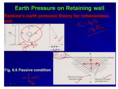
Now talking about the passive condition at that time also we are considering this state of stress okay. So, one soil element we are considering. Here also your sigma h is equal to K p into sigma v which is nothing but K p into gamma into z okay. So, now you see this dotted line is your earth pressure at rest condition that is the variation at earth pressure at rest condition okay. Now this solid line will be giving you the earth pressure at passive state.
