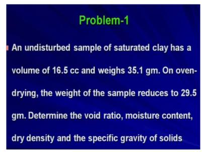
That an undisturbed sample of saturated clay has a volume of 16.5 cc and weighs 35.1 gm. On oven drying the weight of the sample reduces to 29.5 gm. Determine the void ratio, moisture content, dry density, and the specific gravity of solids. So, this problem was taken in the last lecture where we solved the problem by a method, method 1.
