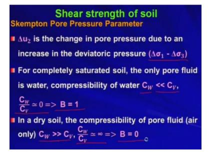
So, delta u 2 is the change in pore water pressure due to an increase in the deviatoric stress or the deviatoric pressure that is delta sigma 1 - delta sigma 3 okay and combine effect will be giving you the total pore pressure increment that is delta u. So, delta u 1 is happening in the first stage delta u 2 is happening in the second stage of the triaxial test and the combination of these 2 will give you the total pore water pressure increment.
