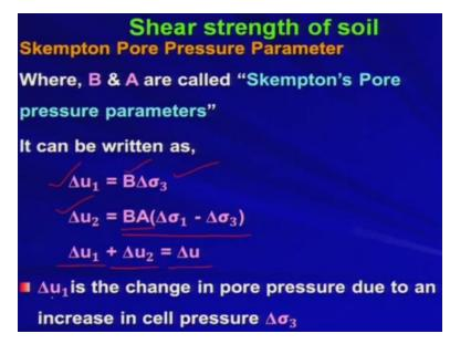
Now from this where B and A are called as Skempton pore pressure parameter. So, now I hope that you have understood that how these 2 parameters are coming into the picture from the basic principle of mechanics okay. So, earlier we introduced that Skempton pore pressure parameters. At that time, we never talked about how these parameters are coming into the picture but now you are quite clear how these parameters are coming into the picture right this B and A.
