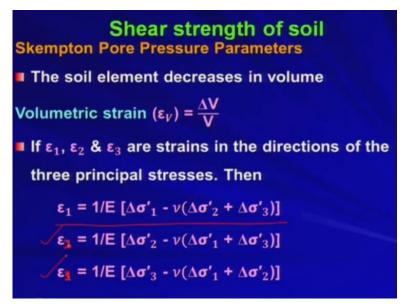
Now under this application of the stress increment you will be getting some volume reduction. That is nothing but the volume volumetric strain. So, the soil element decreases in volume because of the application of the stress increment effective stress increment and that volumetric strain is given by delta V by V where delta V is the volume change and capital V is the original volume okay. So, that is nothing but epsilon V.
