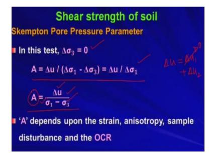
So, in this test delta sigma 3 is 0 what is that consolidated undrained test delta sigma 3 is 0. So, A is nothing but this. So, delta u divided by delta sigma 1. So, what is delta u in this consolidated undrained test because delta u 1 is 0 that is nothing but delta u 2. So, delta u 2 is nothing but your delta u okay. So, from this you can find out A. So, you measured this you know sigma 1 you know sigma 3 you can find out A.
