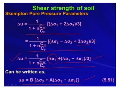
So, if that is so then delta u can be expressed like this from the previous expression which can be further written as this okay delta sigma 1 - delta sigma 3 + 3 into some modification we are doing which can be further written as this what delta u is equal to that is the pore water pressure increment is equal to this.
