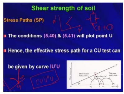
So, the conditions 5.40 and 5.41 will plot point U okay. Hence the effective stress path for a CU test can be given by the curve IU prime U double prime U okay. So, IU prime U double prime U. So, this curve path is your stress path for the CU test agreed. So, how it is moving. So, it is not the straight line now. It is rather the curved line.
