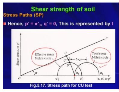
Now hence p prime is equal to sigma 3 prime right and q prime is equal to 0 for this kind of situation okay. So, this is represented by point I so the same point. So, in case of consolidated drained test and in case of consolidated undrained test this point is lying on your p prime axis because that is known as isotropically consolidation consolidated test right. So, all-round you are applying the sigma 3 and then you are consolidating the sample.
