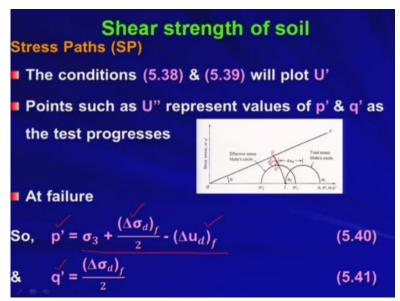
And ultimately the conditions 5.38 and 5.39 will plot U prime. So, points such as U double prime represent values of p prime q prime as the test progresses so as I told you. So, initially you have got U prime then as the test progresses you will be getting another point say U double prime and
