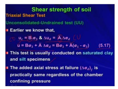
Now earlier we know that u c if you recall whatever we have discussed in case of CD test at that time u c was equal to B into sigma 3 right okay and delta u d is equal to A bar into delta sigma d that is coming from CU test. So, this is coming from CD test so B is the Skempton pore pressure parameter and this is coming from your CU test that is again A bar is your Skempton pore pressure pressure parameter.
