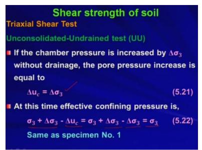
If the chamber pressure is increased by delta sigma 3. So, at sigma 3 we are applying sigma 3 and then we are allowing the allowing the consolidation and we are allowing the pore pressure is becoming zero so with that situation we are starting and then what we are doing we are
