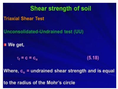
So, therefore we get tau f equal to c only cohesion is equal to Cu where Cu is the undrained shear strength and is equal to the radius of the Mohr circle as you have seen from this figure Cu is nothing but the radius of the Mohr circle. This is your radius okay.
