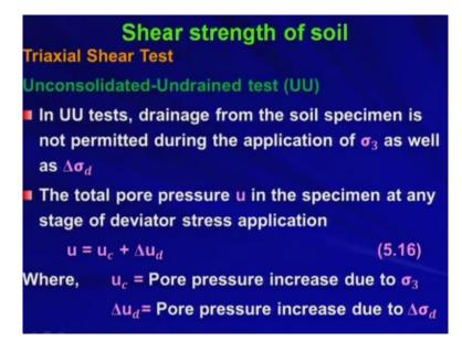
Now coming to the third type of triaxial test that is unconsolidated undrained test that is known as UU test. So, in UU test drainage from the soil specimen is not permitted during the application of sigma 3 as well as delta sigma d. Now what does it mean? So, in case of CD test you allowed drainage okay you allowed consolidation when you applied sigma 3 that means cell pressure and when you applied delta sigma 3 that is deviatoric stress.
