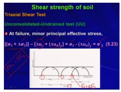
So, at failure minor principle effective stress was sigma 3 plus delta sigma 3 that was the enhanced confining pressure - u c - u d f so why minus, minus delta u c, so why minus delta u c? So, that means this part is getting developed when you increase the confining pressure from sigma 3 to delta sigma 3 right. You did not allow the drainage so it has been developed okay. Now you did not allow the drainage during shearing also. So, therefore at failure delta u d f has
