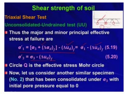
Now thus the major and minor principle effective stress at failure are sigma 1 prime is equal to sigma 3 + delta sigma d f - delta u d f. So, sigma 3 + delta sigma d f is nothing but the total sigma 1 right that is the major principle stress total major principle stress minus the pore water pressure which is getting developed at the failure. So, sigma 1 - delta u d f okay is your sigma 1 prime.
