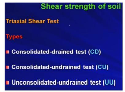
And there we have seen that you have 3 different kinds of say triaxial test one is the consolidated-drained test that is CD test. One is consolidated-undrained test that is CU test and another one is the consolidated unconsolidated-undrained test that is UU test okay.
