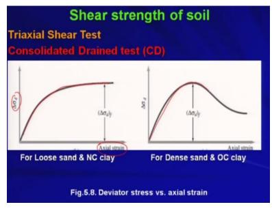
So, now basically we will see that deviatoric stress versus axial strain this plot for loose sand and normally consolidated soil and dense sand and over consolidated soil. It has been seen from the experience and from the test that loose sand and normally consolidated clay will be behaving in a very similar fashion whereas dense sand and over consolidated clay will be behaving in a very similar fashion.
