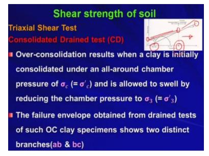
So, over consolidation results when a clay is initially consolidated under an all-round chamber pressure of sigma c and which is eventually equal to sigma c prime because the total stress and the effective stress both are equal or both are same in case of CD test right because you are allowing the drainage so there is no excess pore water pressure getting built up. So, the pore water pressure is zero.
