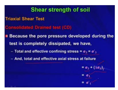
Now because the pore pressure developed during the test is completely dissipated right so there is no excess pore water pressure. So, the pore pressure developed whatever pore pressure was getting developed inside the soil specimen due to the application of sigma 3 alone and then sigma 3 plus delta sigma d along the axial direction so whatever is the situation whatever is the condition you have allowed the drainage so therefore no pore pressure is getting built up right.
