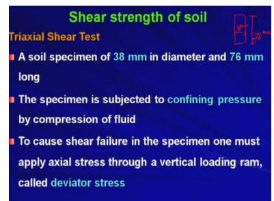
So, a soil specimen in this physical test what we consider we consider some cylindrical soil specimen. The soil specimen of 38 mm in diameter and 76 mm long generally we consider this kind of soil specimen so we have to I mean we have to do some P test say exercise okay so to prepare the soil. So, basically the sample should be made of some cylindrical sample something like this okay so 38 mm diameter and 76 mm height okay.
