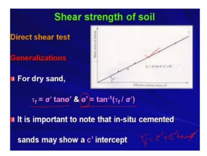
Now for dry sand, so already we have seen so tau f is equal to sigma prime tan phi prime. Therefore, phi prime is nothing but tan inverse tau f by sigma prime. So, after establishing this line you can get the inclination of this line with the sigma axis and which is nothing but phi prime. So, now you can use this phi prime for your design purpose.
