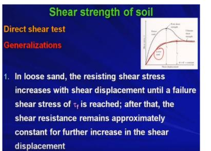
Now in loose sand so now we are going to discuss this stress strain behaviour for loose sand as well as the dense sand. So, in loose sand the resisting shear stress increases with shear
