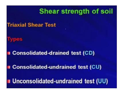
Now what are the different types of triaxial test? The first one is consolidated-drained test okay. We will come to these tests individually and we will discuss the pros and cons of each test and we will see that what are the different procedure you have to follow to obtain these different types of triaxial test. The first one is consolidated-drained test. Generally, it is defined or it is represented as CD test okay in soil mechanics.
