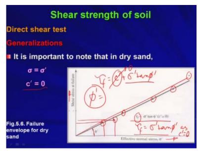
Now it is important to know that in dry sand if you consider the dry sand right completely dry sand there is no water at all so sigma is nothing but the sigma prime that is the total stress is must be equal to the effective stress because only water will cause the difference between the total stress and the effective stress. If water is not there at all then the total stress must be equal to the effective stress and c prime that is the cohesion that is the effective cohesion must be zero.
